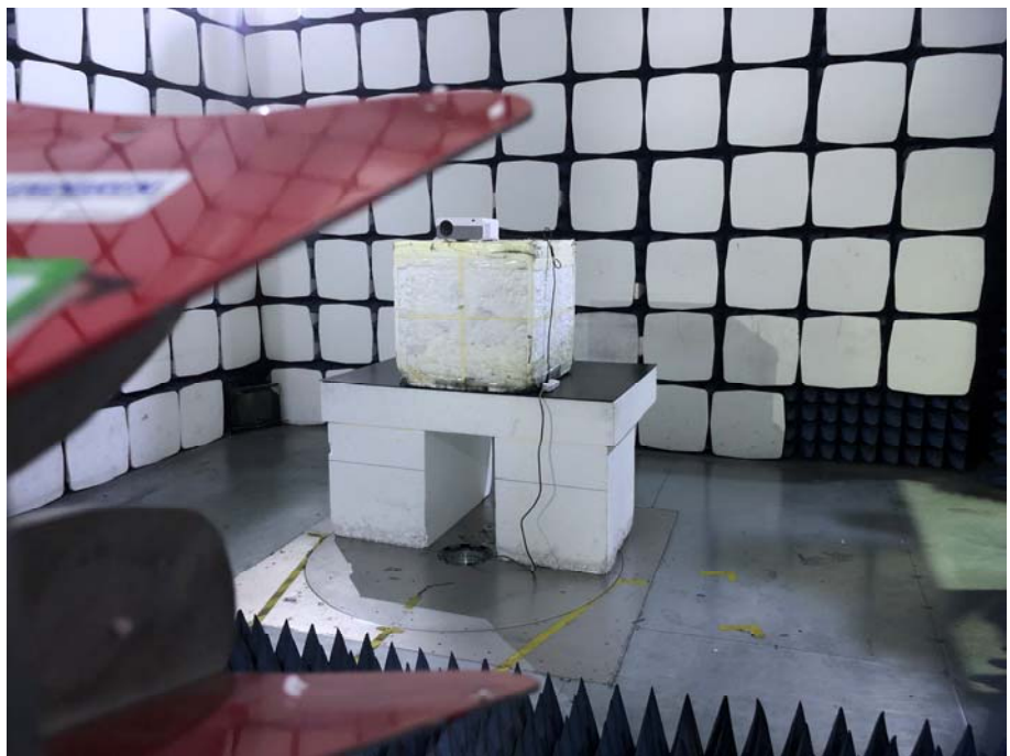
Radiation Emission Test Setup (1GHz to 18GHz)
