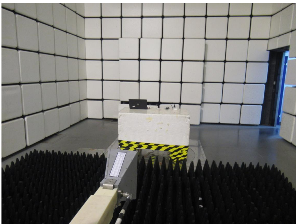
Picture 1 Radiated Emission Test Setup
