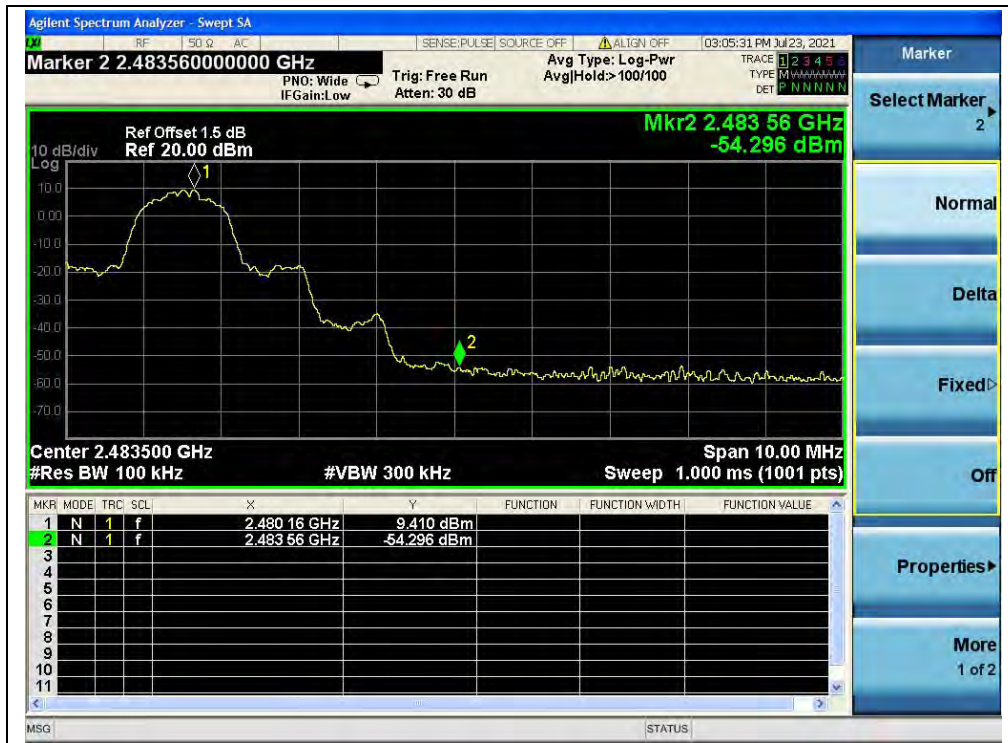
(Band edge, Channel 78, \pi/4 -DQPSK)
