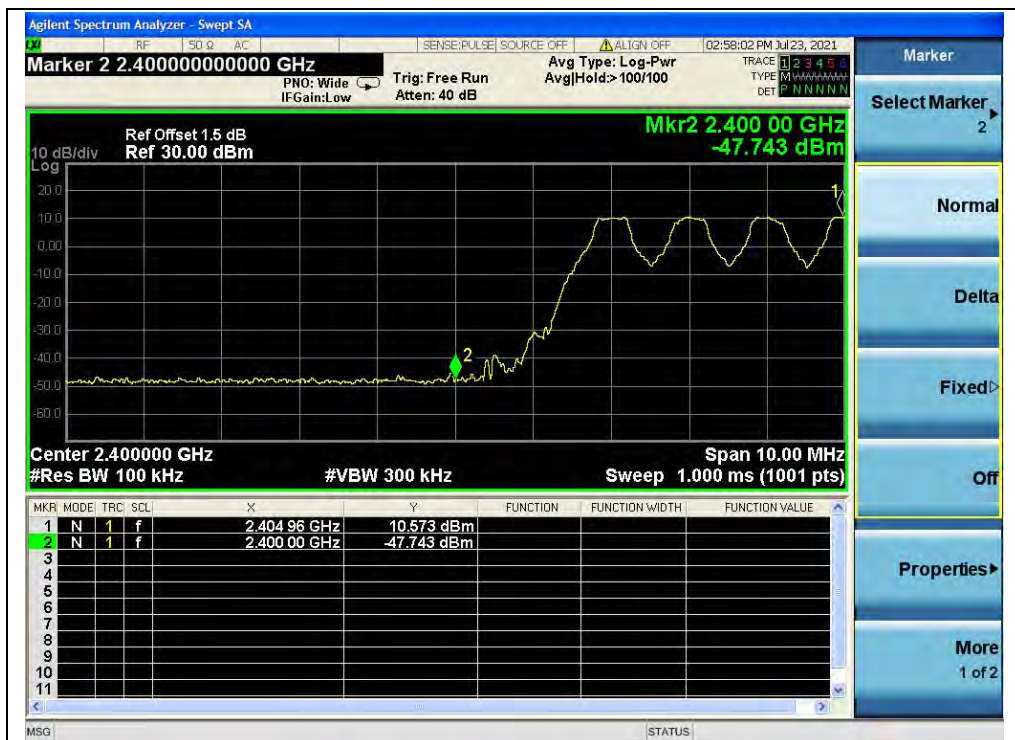
(Band edge with hopping on, Channel 0, GFSK)
