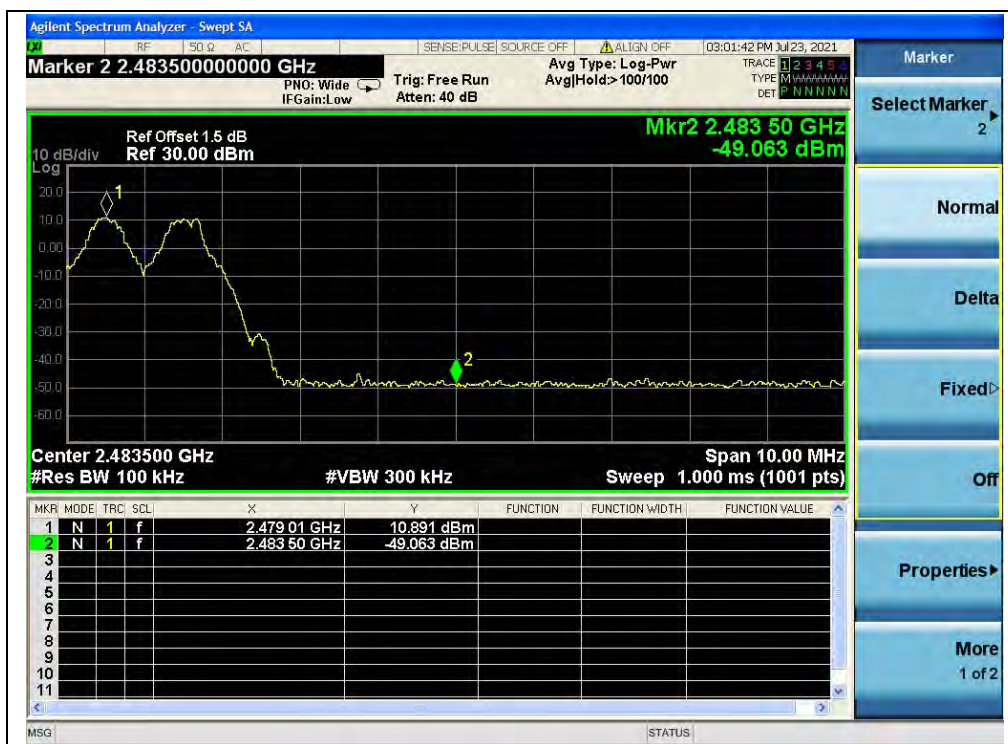
(Band edge with hopping on, Channel 78, GFSK)
