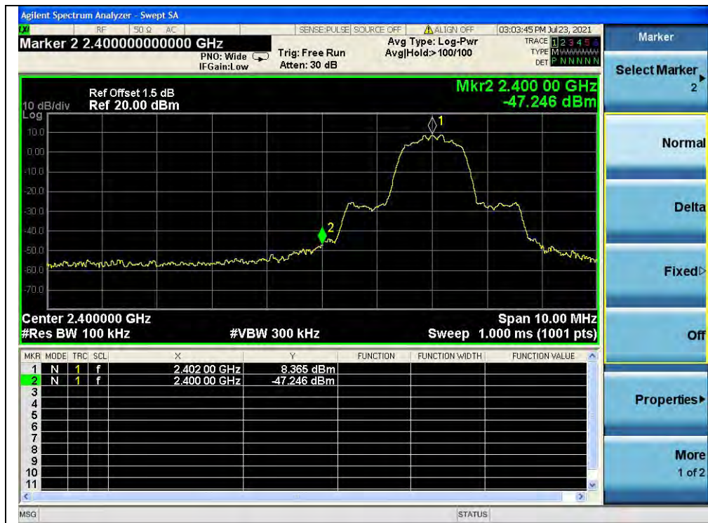
(Band edge, Channel 0, \pi/4 -DQPSK)
