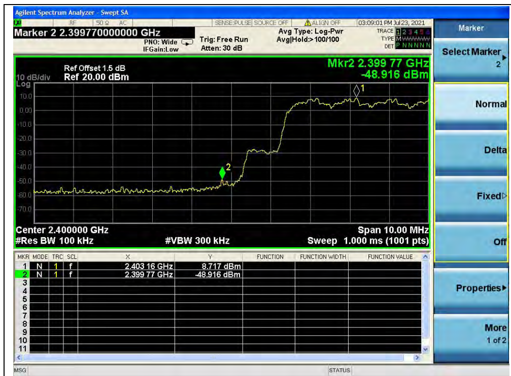
(Band edge with hopping on, Channel 0, 8-DPSK)
