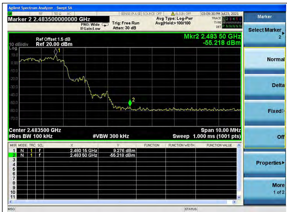
(Band edge with hopping on, Channel 78, 8-DPSK)
