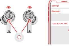
ADDING NEW/ADDITIONAL BLUETOOTH DEVICES: Turn OFF Bluetooth from any previously connected device. Turn ON Bluetooth from new device. Take earbuds out of the case. Earbuds will automatically enter Bluetooth Pairing. Select "JLab Epic Air ANC" in new device settings to connect.
