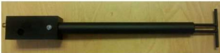
**Figure 1 – MVG COMOSAR Validation Dipole**
