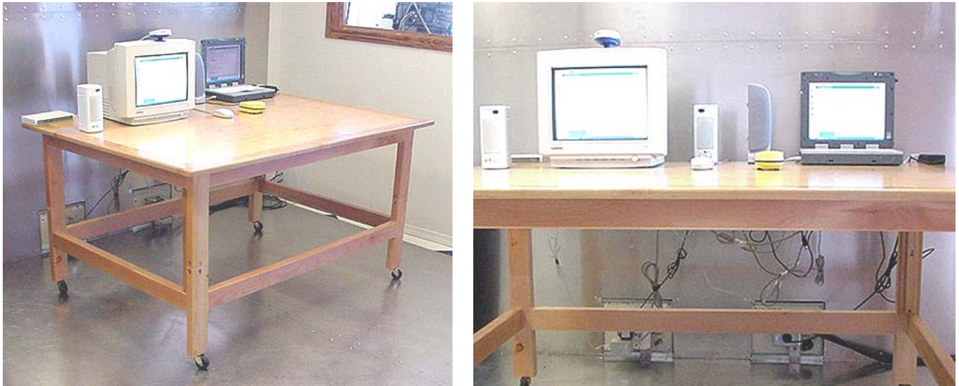
Photograph H-2 – AC Powerline Conducted Emission Cable Placement
