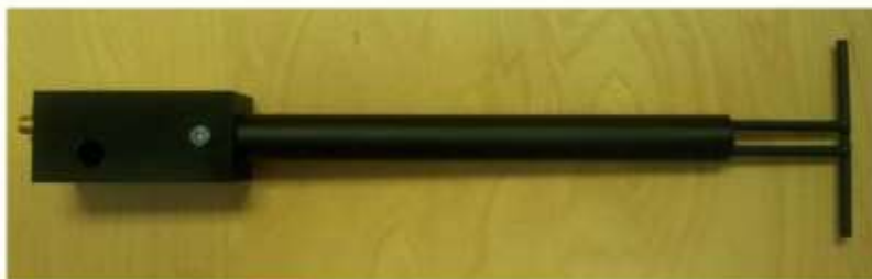
Figure 1 – MVG COMOSAR Validation Dipole
