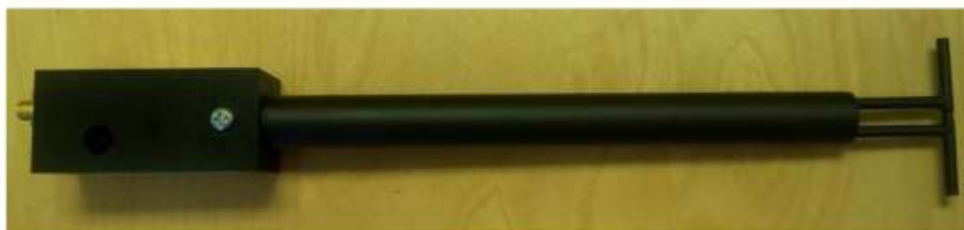
Figure 1 – MVG COMOSAR Validation Dipole
