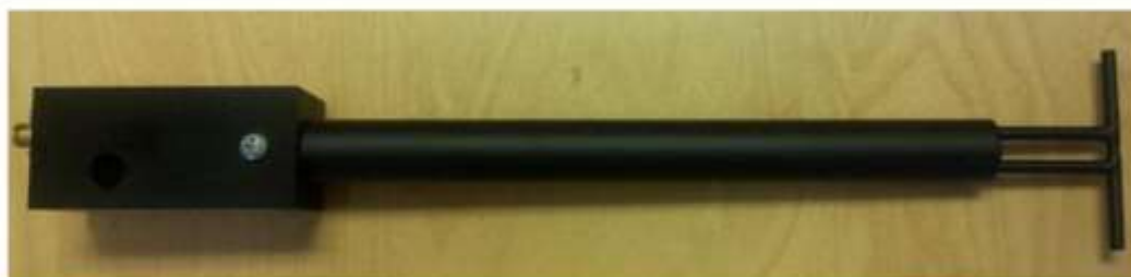
Figure 1 – MVG COMOSAR Validation Dipole
