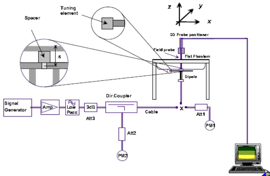
With the SG and Amp and with directional coupler in place, set up the source signal at the relevant frequency and use a power meter to measure the power at the end of the SMA cable that you intend to connect to the balanced dipole. Adjust the SG to make this, say, 0.01W (10 dBm). If this level is too high to read directly with the power meter sensor, insert a calibrated attenuator (e.g. 10 or 20 dB) and make a suitable correction to the power meter reading.
