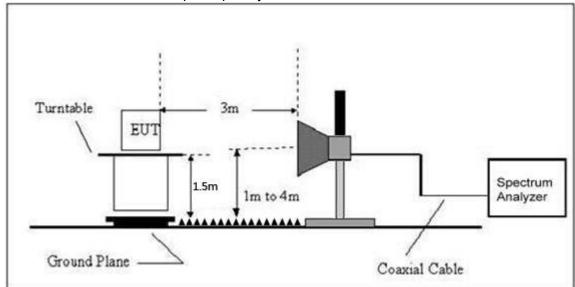
(C) Radiated Emission Test-Up Frequency Above 1GHz
