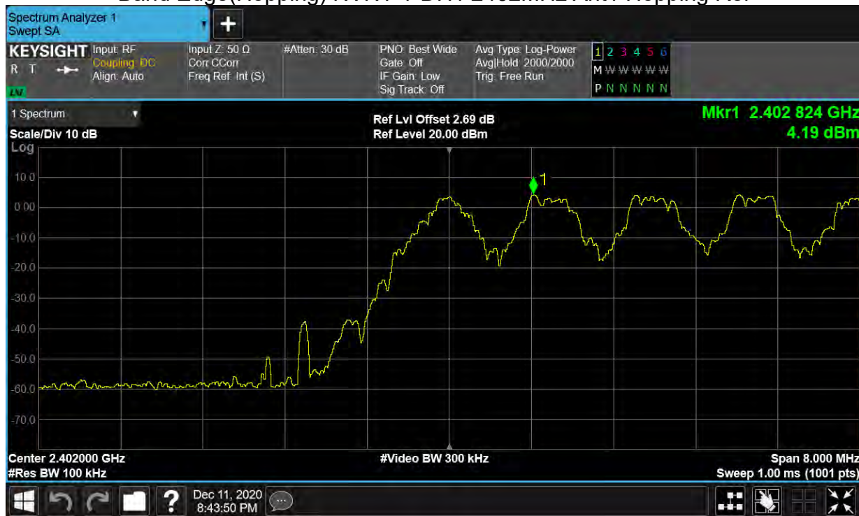
Band Edge(Hopping) NVNT 1-DH1 2402MHz Ant1 Hopping Emission
