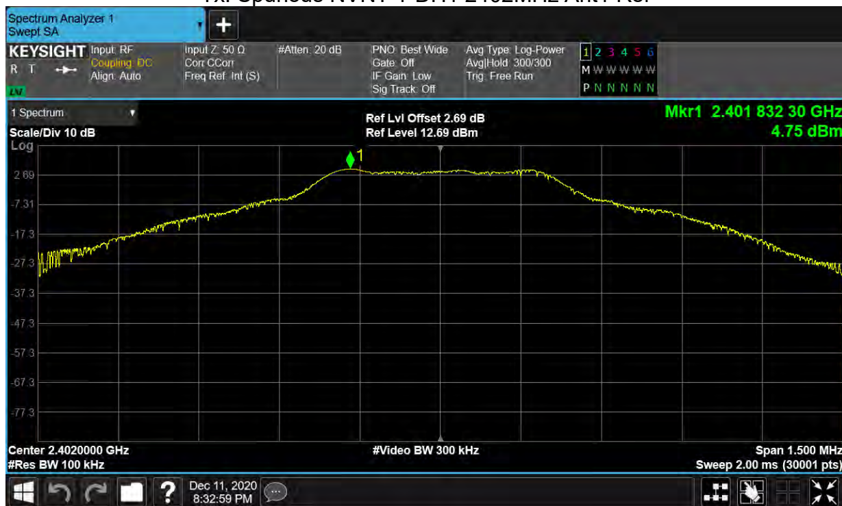
Tx. Spurious NVNT 1-DH1 2402MHz Ant1 Emission
