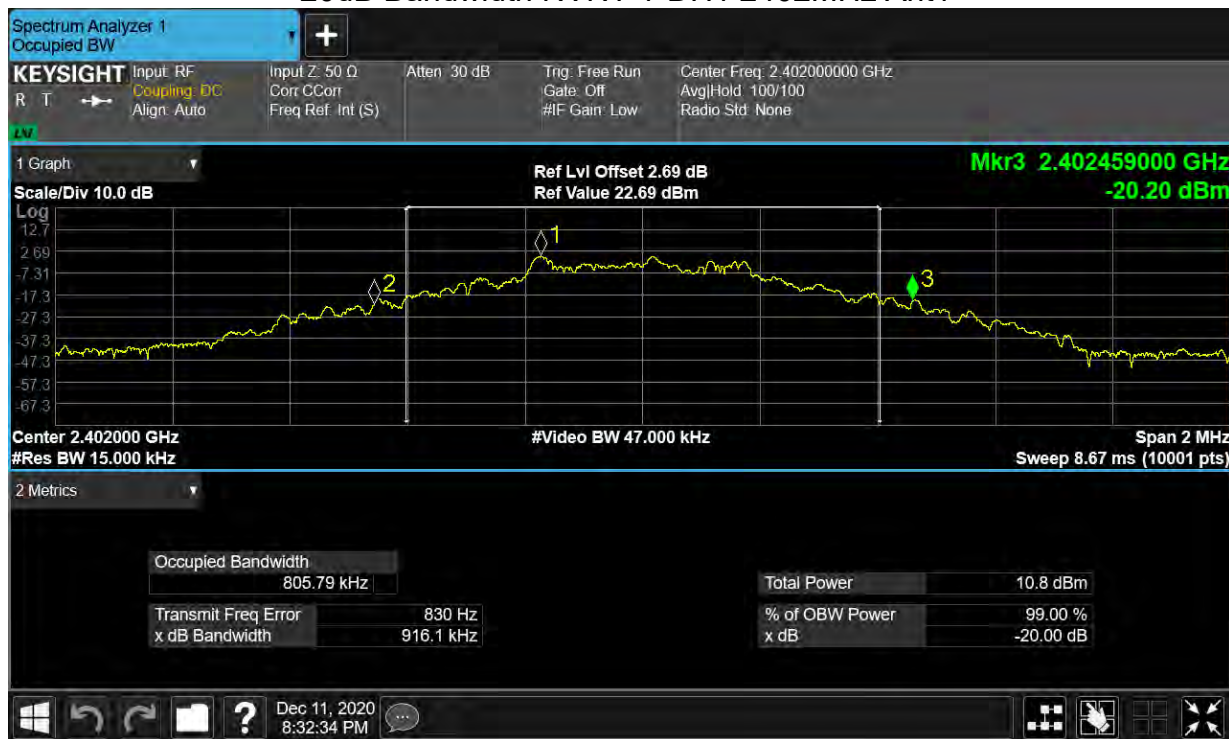
-20dB Bandwidth NVNT 1-DH1 2402MHz Ant1
