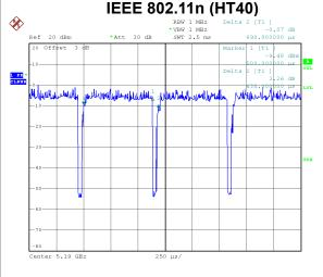
Duty cycle = 1.300 ms / 1.345 ms = 96.65 %Duty Factor =  $10 * \log(1 / 96.65\%) = 0.15 \text{ dB}$
