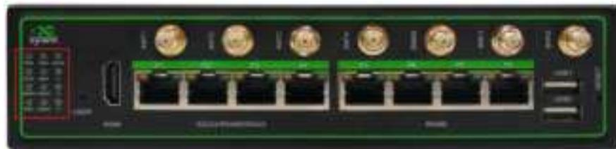
EC954-FQ38 has 12 LED lights that respectively indicate the power supply and system operation status.
