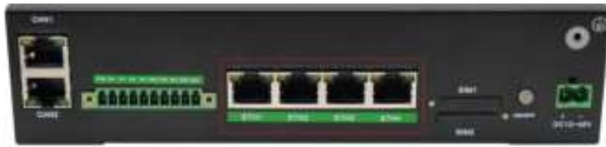
EC954-FQ38 has four RJ45 Ethernet ports and supports 10M/100M/1000M adaptive rates.
