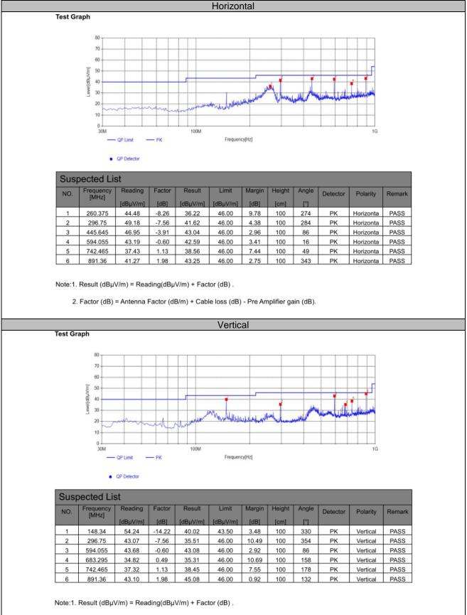
2. Factor (dB) = Antenna Factor (dB/m) + Cable loss (dB) - Pre Amplifier gain (dB).
