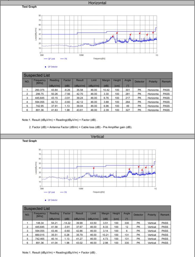
2. Factor (dB) = Antenna Factor (dB/m) + Cable loss (dB) - Pre Amplifier gain (dB).
