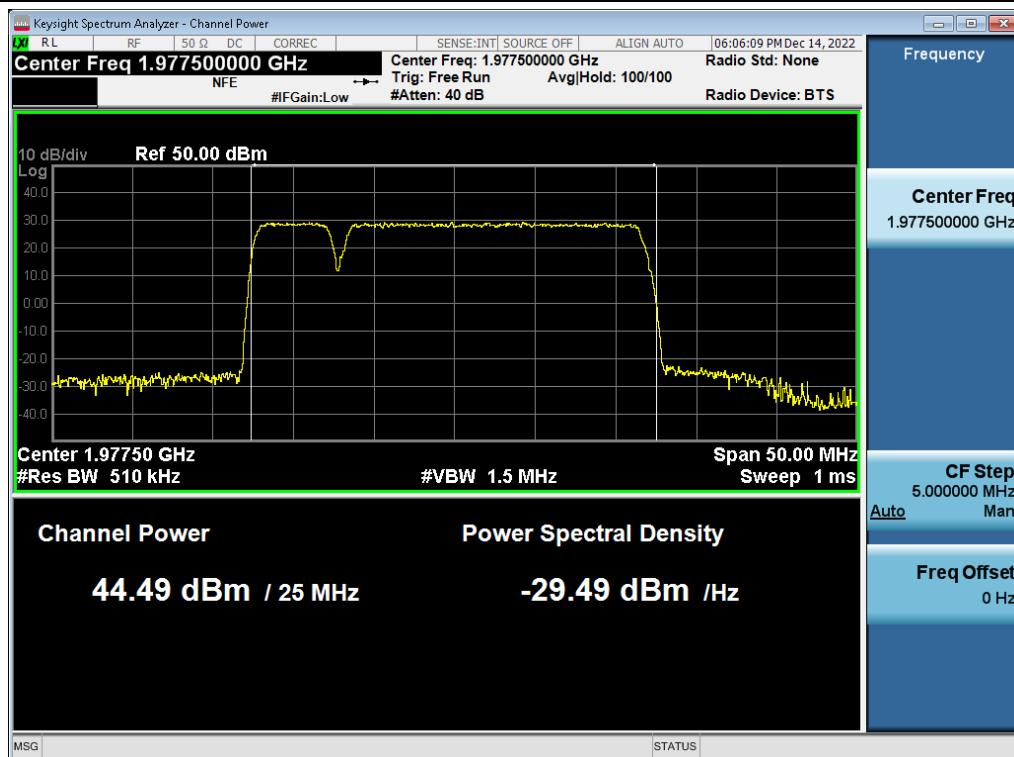
**Antenna 2 / (4 Port) LTE B2 5 MHz 1 Carrier + 5G NR n2 5 MHz 1 Carrier + DSS B2 20 MHz 1 Carrier [3 Carrier] [2C+1C] / LTE B2 5 MHz 1 Carrier + 5G NR n2 5 MHz 1 Carrier / 256QAM / Low / Non-Contiguous**
