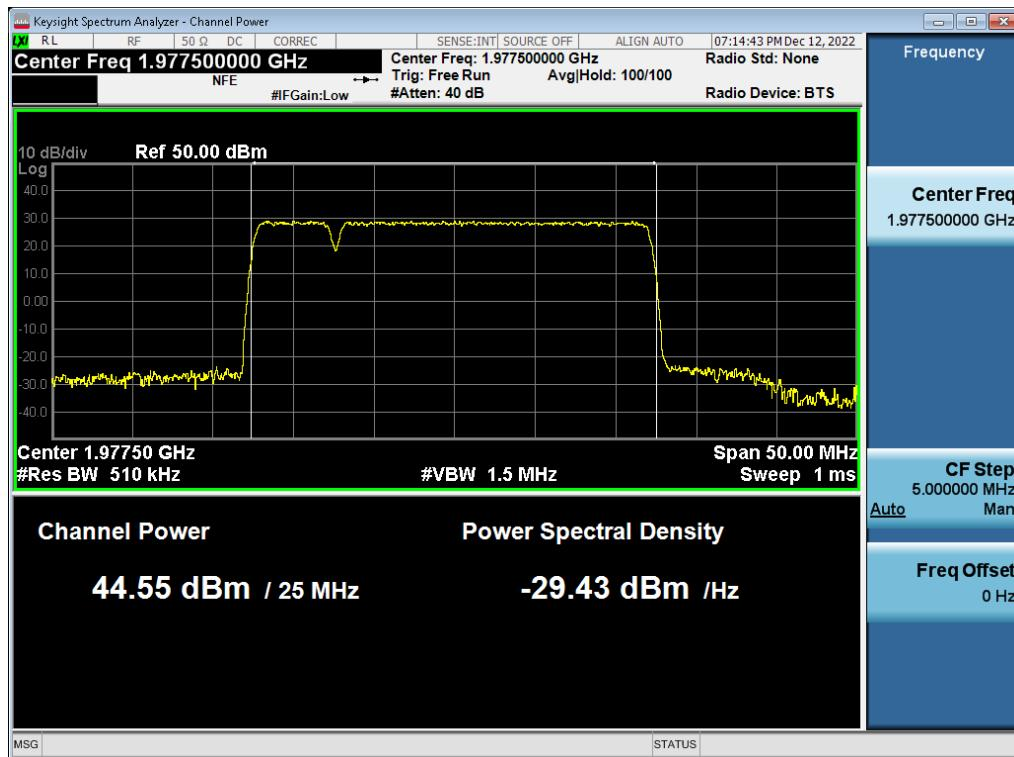
**Antenna 2 / (4 Port) 5G NR n2 5 MHz 1 Carrier + 5G NR n2 5 MHz 1 Carrier + 5G NR n2 20 MHz 1 Carrier [3 Carrier]
