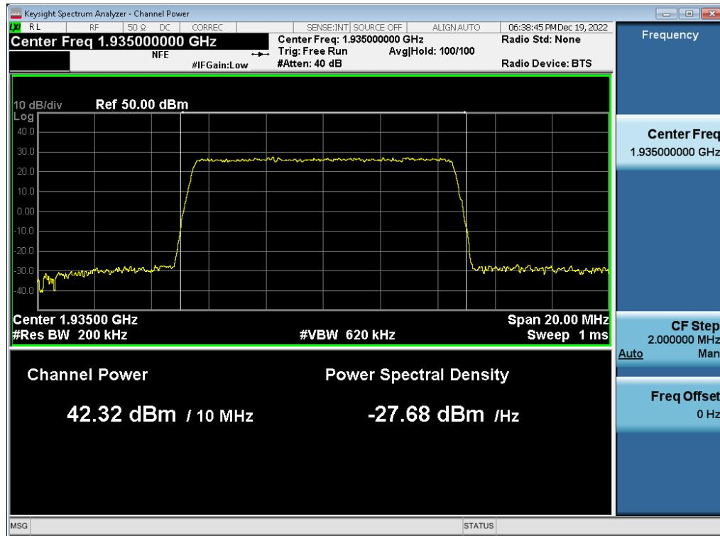
**Antenna 1 / (2 Port) DSS B2 10 MHz 1 Carrier + DSS B2 10 MHz 1 Carrier + DSS B2 10 MHz 1 Carrier [3 Carrier] [1C+2C] / DSS B2 10 MHz 1 Carrier + DSS B2 10 MHz 1 Carrier / 64QAM / High / Non-Contiguous**
