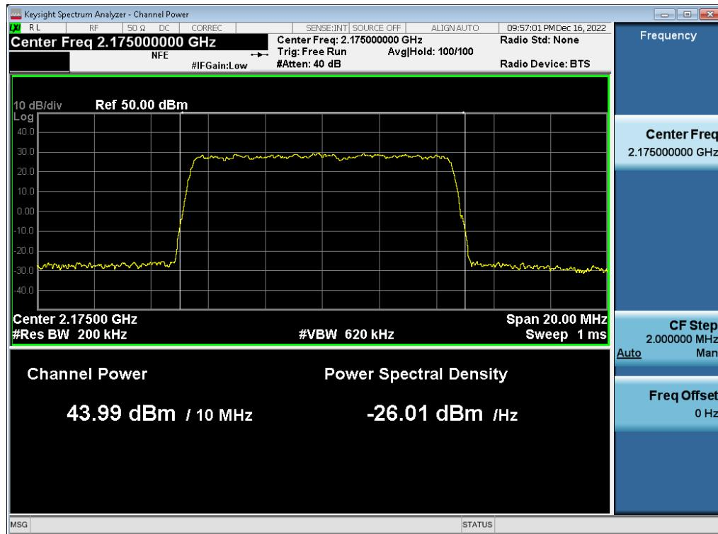
**Antenna 1 / (2 Port) LTE B66 5 MHz 1 Carrier + LTE B66 5 MHz 1 Carrier + DSS B66 10 MHz 1 Carrier + DSS B66 20 MHz 1 Carrier [4 Carrier] [1C+3C] / LTE B66 5 MHz 1 Carrier / 256QAM / Low / Non-Contiguous**
