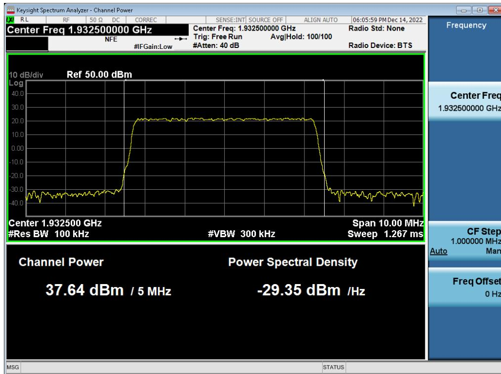
Antenna 2 / (4 Port) LTE B2 5 MHz 1 Carrier + 5G NR n2 5 MHz 1 Carrier + DSS B2 20 MHz 1 Carrier [3 Carrier] [1C+2C] /
