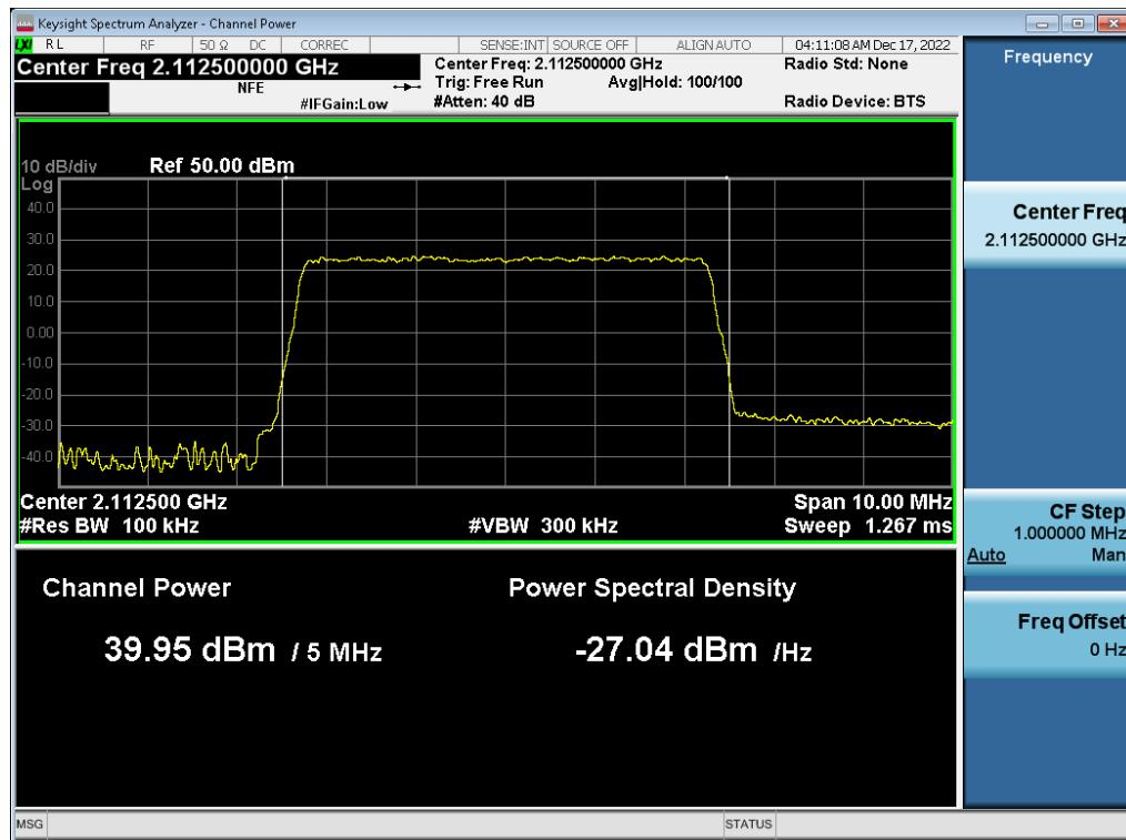
**Antenna 1 / (2 Port) LTE B66 5 MHz 1 Carrier + LTE B66 5 MHz 1 Carrier + DSS B66 10 MHz 1 Carrier + DSS B66 20 MHz 1 Carrier [4 Carrier] [1C+3C] / LTE B66 5 MHz 1 Carrier + DSS B66 10 MHz 1 Carrier + DSS B66 20 MHz 1 Carrier / 256QAM / High / Non-Contiguous**
