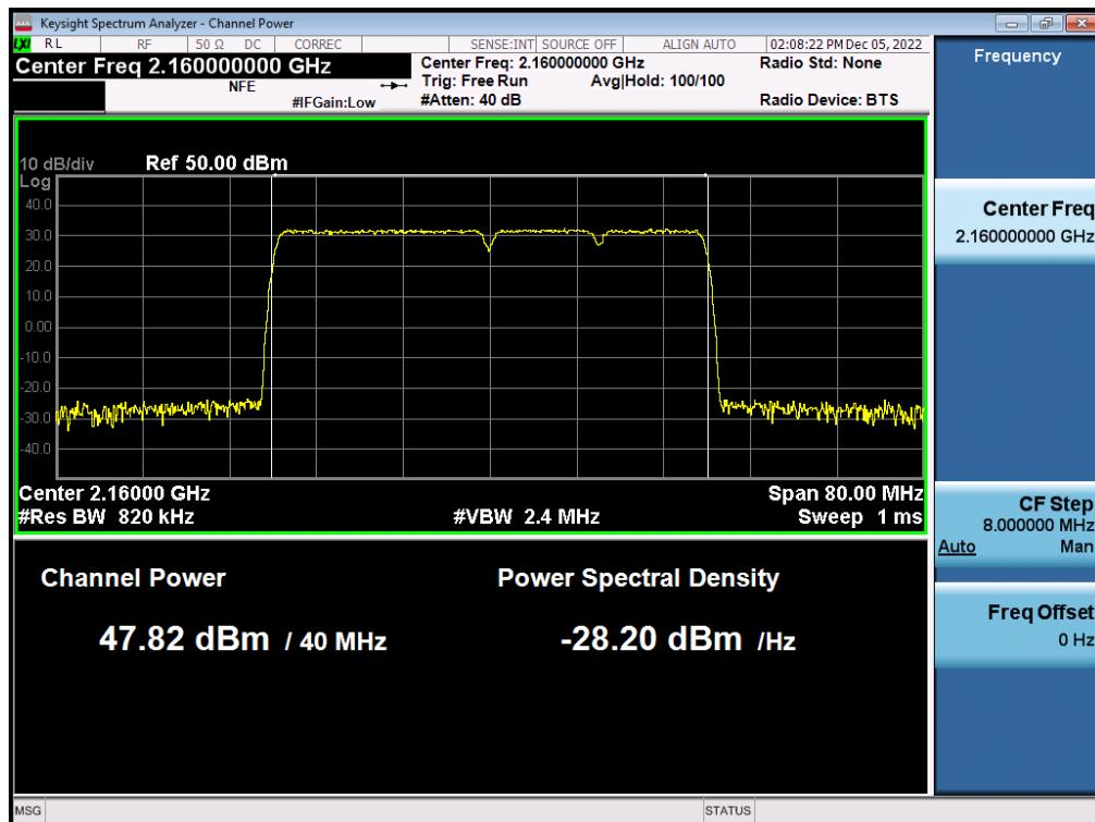
**Antenna 1 / (4 Port) 5G NR n66 5 MHz 1 Carrier + 5G NR n66 5 MHz 1 Carrier + DSS B66 10 MHz 1 Carrier [3 Carrier] / 64QAM / High / Contiguous**
