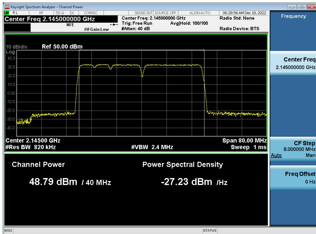
**Antenna 1 / (2 Port) LTE B66 5 MHz 1 Carrier + LTE B66 5 MHz 1 Carrier + DSS B66 10 MHz 1 Carrier + DSS B66 10 MHz 1 Carrier [4 Carrier] / 256QAM / Middle / Contiguous**
