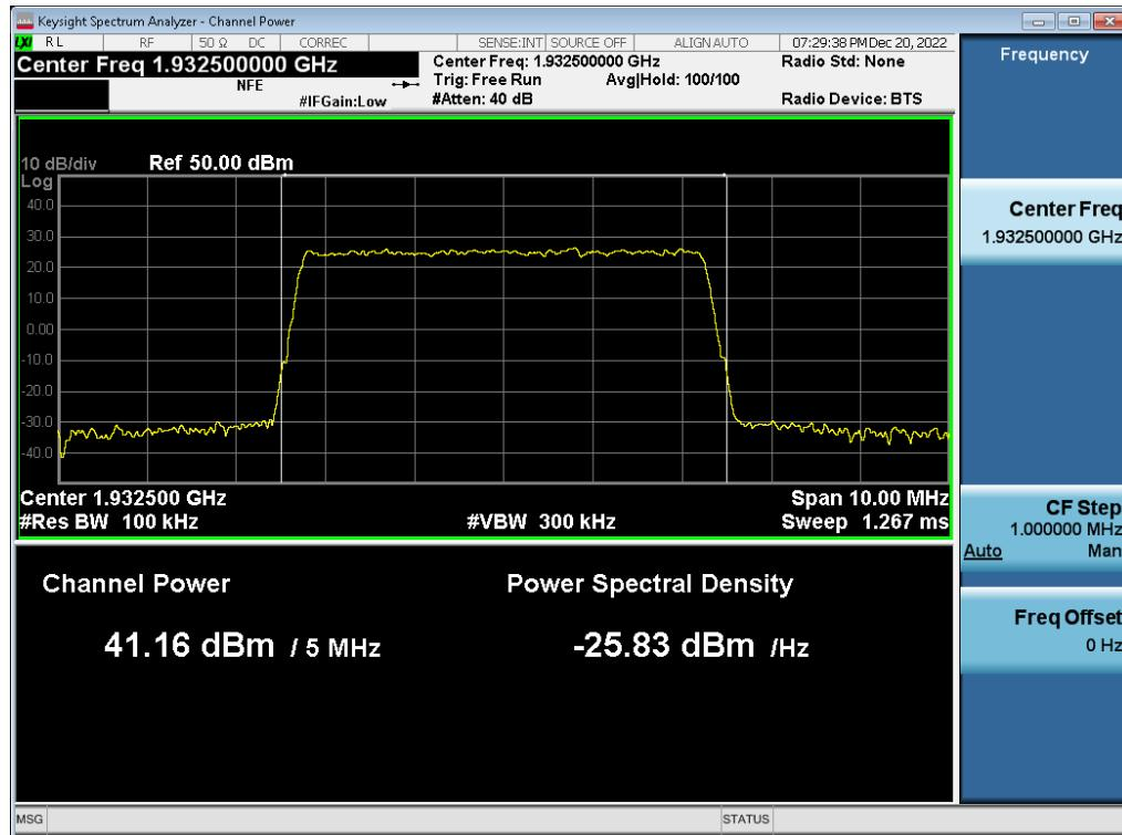
**Antenna 1 / (2 Port) 5G NR n2 5 MHz 1 Carrier + 5G NR n2 5 MHz 1 Carrier + DSS B2 10 MHz 1 Carrier [3 Carrier] [1C+2C] / 5G NR n2 5 MHz 1 Carrier + DSS B2 10 MHz 1 Carrier / 256QAM / High / Non-Contiguous**
