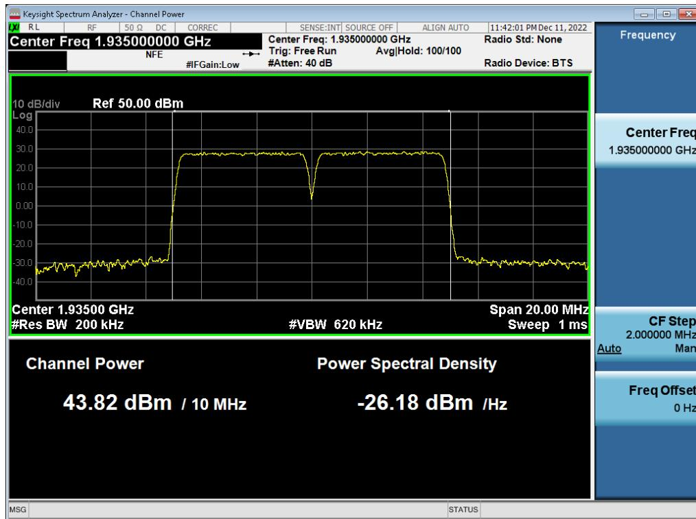
**Antenna 2 / (4 Port) 5G NR n2 5 MHz 1 Carrier + 5G NR n2 5 MHz 1 Carrier + 5G NR n2 5 MHz 1 Carrier [3 Carrier] [2C+1C]
