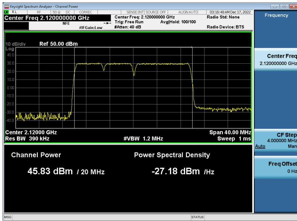
**Antenna 1 / (2 Port) LTE B66 5 MHz 1 Carrier + LTE B66 5 MHz 1 Carrier + DSS B66 10 MHz 1 Carrier + DSS B66 20 MHz 1 Carrier [4 Carrier] [3C+1C] / DSS B66 20 MHz 1 Carrier / 256QAM / High / Non-Contiguous**
