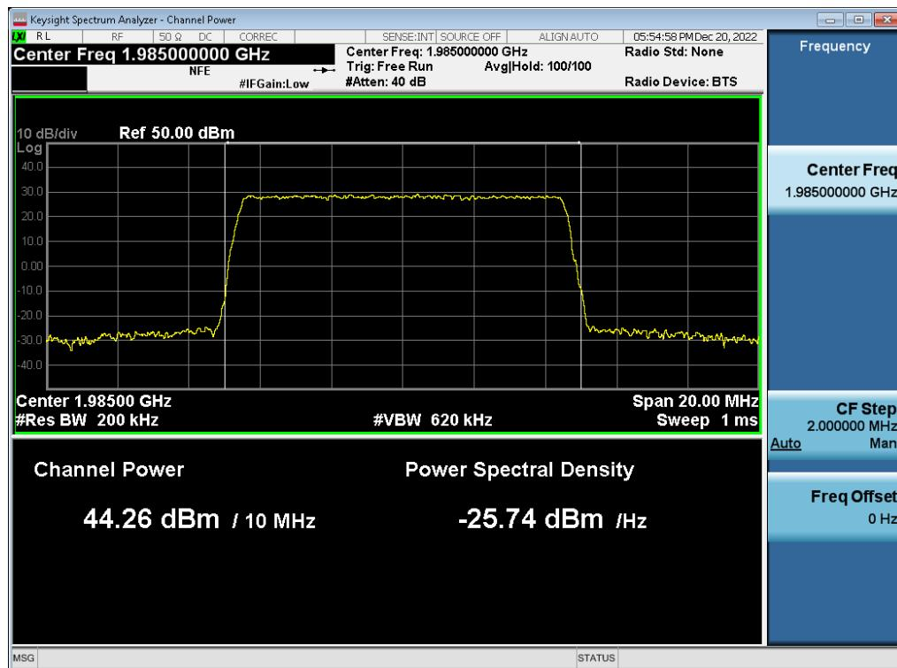
**Antenna 1 / (2 Port) 5G NR n2 5 MHz 1 Carrier + 5G NR n2 5 MHz 1 Carrier + DSS B2 20 MHz 1 Carrier [3 Carrier] [1C+2C] / 5G NR n2 5 MHz 1 Carrier / 256QAM / Low / Non-Contiguous**
