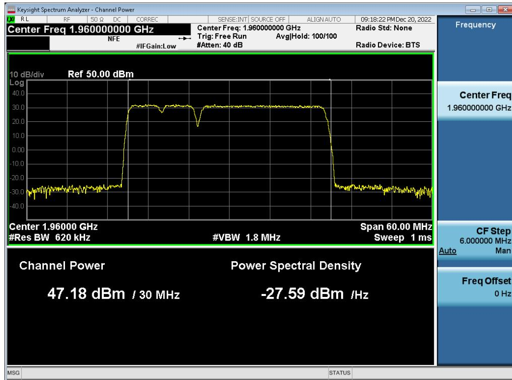
**Antenna 0 / (2 Port) DSS B2 10 MHz 1 Carrier + DSS B2 10 MHz 1 Carrier + DSS B2 10 MHz 1 Carrier [3 Carrier] / 64QAM / Low / Contiguous**
