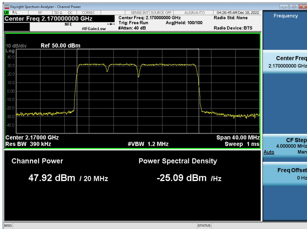
**Antenna 1 / (2 Port) LTE B66 5 MHz 1 Carrier + 5G NR n66 5 MHz 1 Carrier + 5G NR n66 5 MHz 1 Carrier + DSS B66 10 MHz 1 Carrier [4 Carrier] [3C+1C] / LTE B66 5 MHz 1 Carrier + 5G NR n66 5 MHz 1 Carrier + 5G NR n66 5 MHz 1 Carrier / 256QAM / Low / Non-Contiguous**
