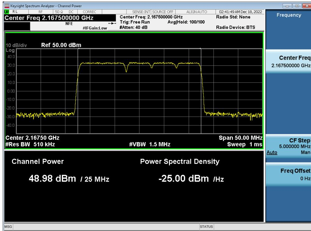
**Antenna 1 / (2 Port) LTE B66 5 MHz 1 Carrier + 5G NR n66 5 MHz 1 Carrier + DSS B66 10 MHz 1 Carrier + DSS B66 20 MHz 1 Carrier [4 Carrier] / 256QAM / Middle / Contiguous**
