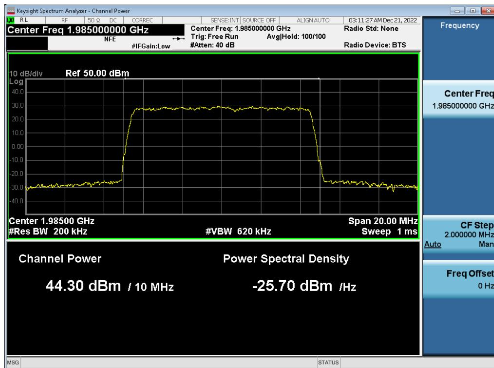
**Antenna 1 / (2 Port) LTE B2 5 MHz 1 Carrier + 5G NR n2 5 MHz 1 Carrier + DSS B2 20 MHz 1 Carrier [3 Carrier] [1C+2C] / LTE B2 5 MHz 1 Carrier / 256QAM / Low / Non-Contiguous**
