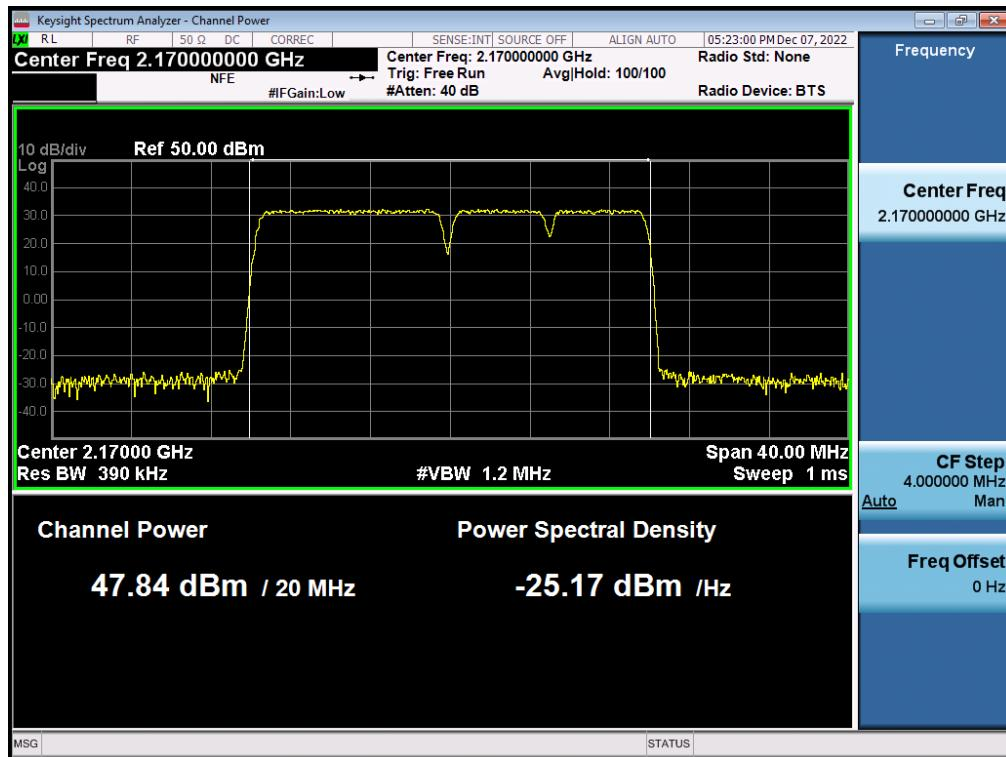
**Antenna 1 / (4 Port) 5G NR n66 10 MHz 1 Carrier + 5G NR n66 20 MHz 1 Carrier + DSS B66 10 MHz 1 Carrier [3 Carrier] / 64QAM / Middle / Contiguous**
