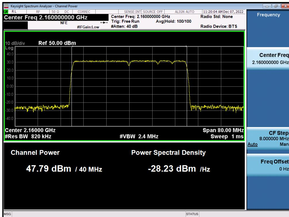
**Antenna 1 / (4 Port) LTE B66 5 MHz 1 Carrier + 5G NR n66 5 MHz 1 Carrier + 5G NR n66 5 MHz 1 Carrier + DSS B66 10 MHz 1 Carrier [4 Carrier] / 16QAM / High / Contiguous**
