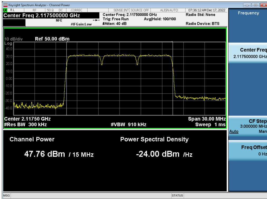
**Antenna 1 / (2 Port) LTE B66 5 MHz 1 Carrier + 5G NR n66 5 MHz 1 Carrier + 5G NR n66 5 MHz 1 Carrier + 5G NR n66 5 MHz 1 Carrier [4 Carrier] [3C+1C] / 5G NR n66 5 MHz 1 Carrier / 256QAM / High / Non-Contiguous**
