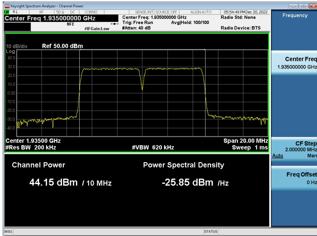
**Antenna 1 / (2 Port) 5G NR n2 5 MHz 1 Carrier + 5G NR n2 5 MHz 1 Carrier + DSS B2 10 MHz 1 Carrier [3 Carrier] [2C+1C] / DSS B2 10 MHz 1 Carrier / QPSK / High / Non-Contiguous**
