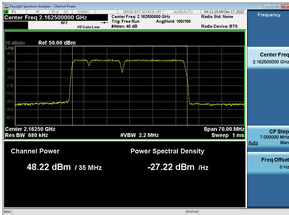
**Antenna 1 / (2 Port) LTE B66 5 MHz 1 Carrier + LTE B66 5 MHz 1 Carrier + DSS B66 10 MHz 1 Carrier + DSS B66 20 MHz 1 Carrier [4 Carrier] [3C+1C] / LTE B66 5 MHz 1 Carrier + LTE B66 5 MHz 1 Carrier + DSS B66 10 MHz 1 Carrier / 256QAM / Low / Non-Contiguous**
