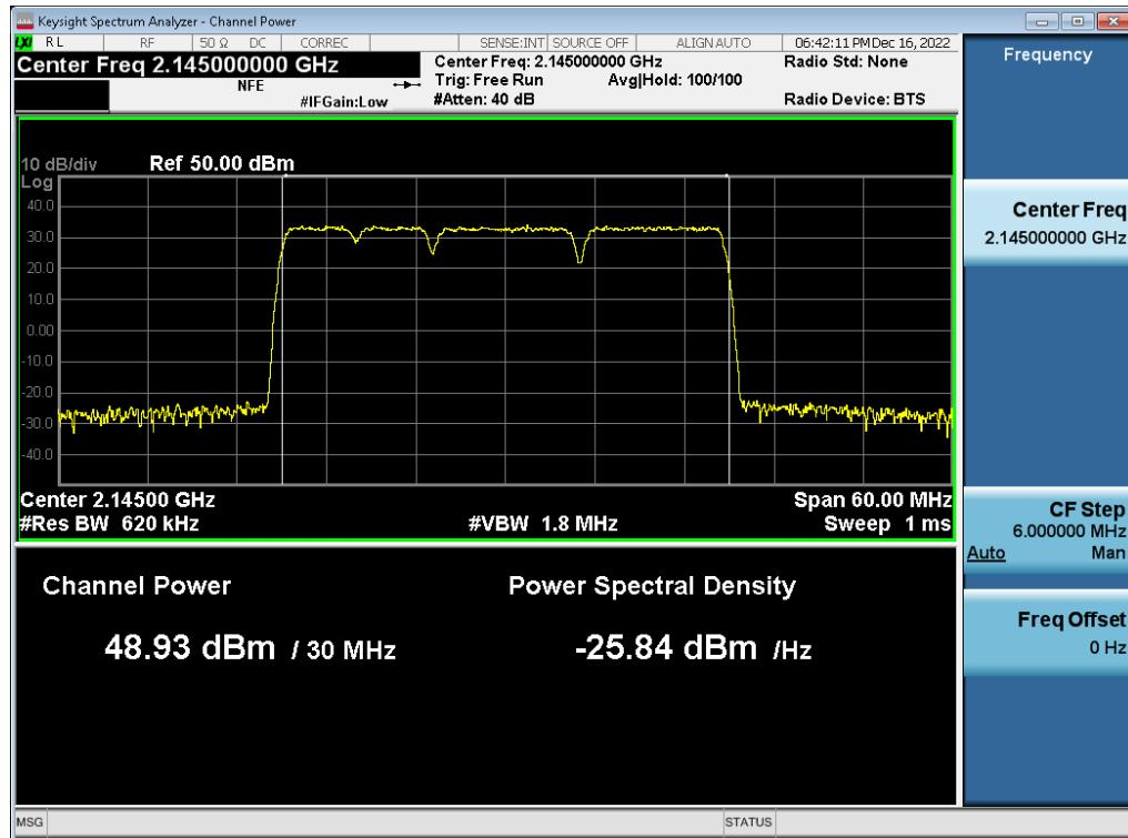
**Antenna 1 / (2 Port) LTE B66 5 MHz 1 Carrier + LTE B66 5 MHz 1 Carrier + DSS B66 10 MHz 1 Carrier + DSS B66 20 MHz 1 Carrier [4 Carrier] / 256QAM / High / Contiguous**
