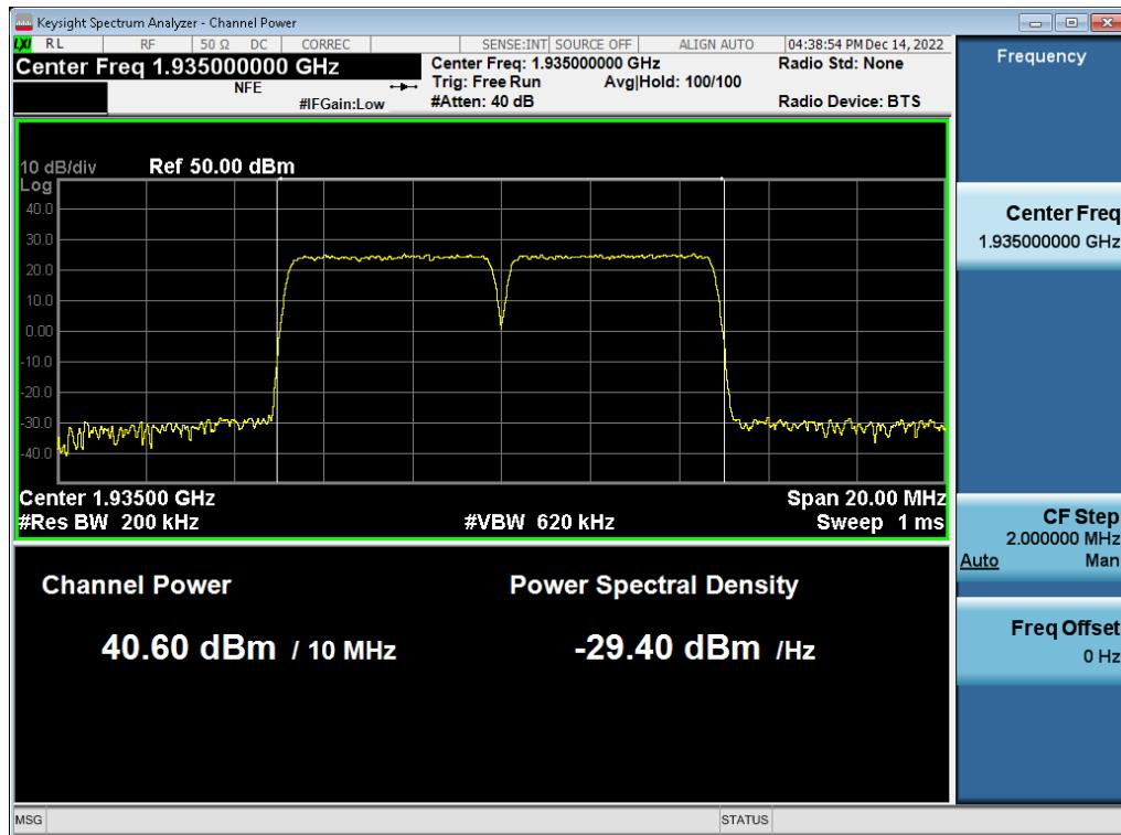
**Antenna 2 / (4 Port) LTE B2 5 MHz 1 Carrier + 5G NR n2 5 MHz 1 Carrier + DSS B2 20 MHz 1 Carrier [3 Carrier] [2C+1C] / DSS B2 20 MHz 1 Carrier / 256QAM / High / Non-Contiguous**
