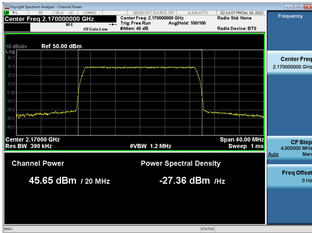
**Antenna 1 / (2 Port) LTE B66 5 MHz 1 Carrier + LTE B66 5 MHz 1 Carrier + DSS B66 10 MHz 1 Carrier + DSS B66 10 MHz 1 Carrier [4 Carrier] [1C+3C] / LTE B66 5 MHz 1 Carrier / 256QAM / Low / Non-Contiguous**
