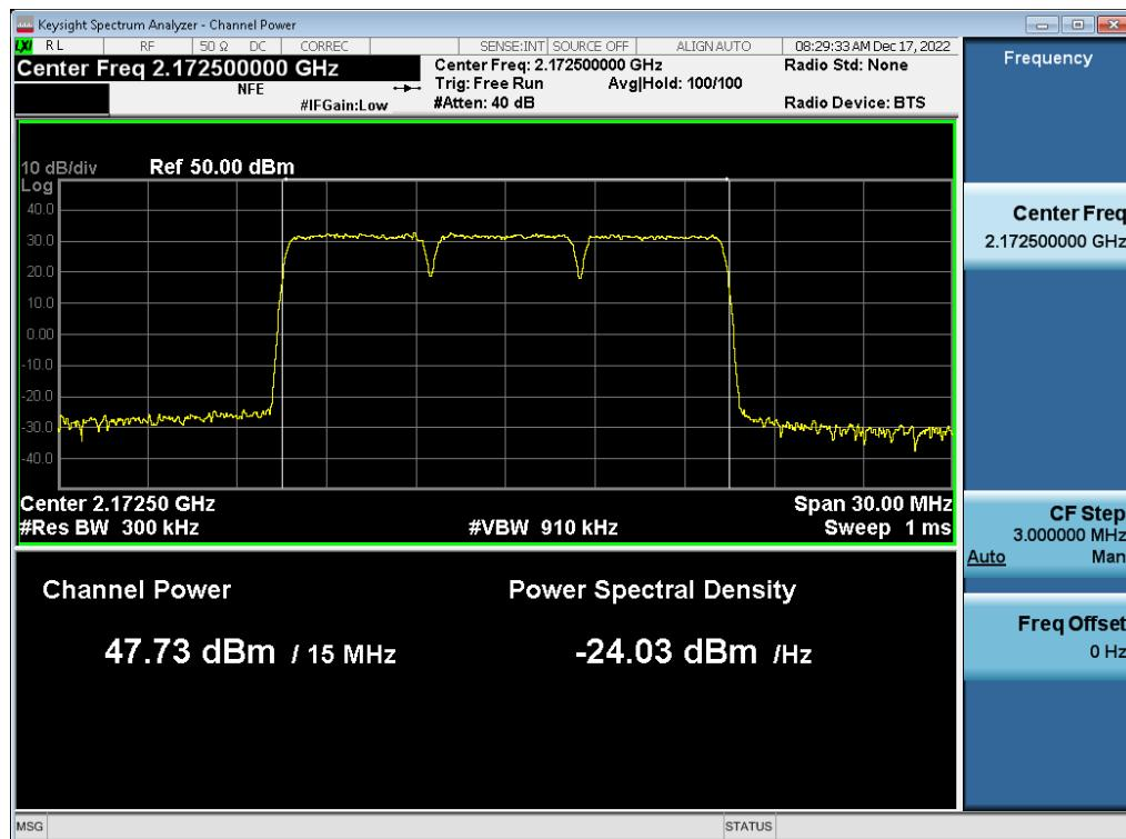
**Antenna 1 / (2 Port) LTE B66 5 MHz 1 Carrier + 5G NR n66 5 MHz 1 Carrier + 5G NR n66 5 MHz 1 Carrier + 5G NR n66 5 MHz 1 Carrier [4 Carrier] [3C+1C] / LTE B66 5 MHz 1 Carrier + 5G NR n66 5 MHz 1 Carrier + 5G NR n66 5 MHz 1 Carrier / 256QAM / Low / Non-Contiguous**
