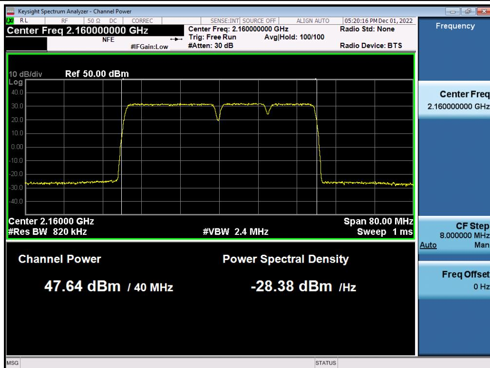
**Antenna 1 / (4 Port) LTE B66 5 MHz 1 Carrier + 5G NR n66 5 MHz 1 Carrier + 5G NR n66 5 MHz 1 Carrier + 5G NR n66 5 MHz 1 Carrier [4 Carrier] / 64QAM / Middle / Contiguous**
