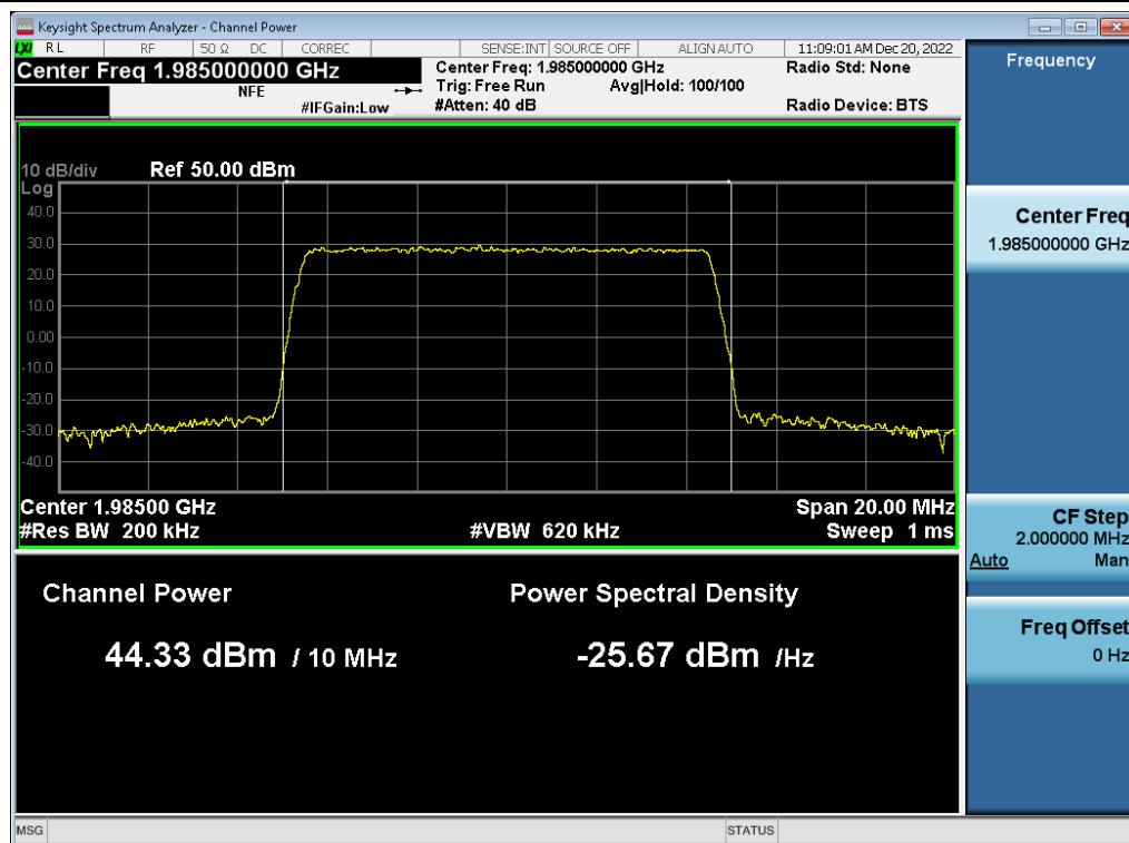
**Antenna 1 / (2 Port) LTE B2 5 MHz 1 Carrier + 5G NR n2 5 MHz 1 Carrier + DSS B2 10 MHz 1 Carrier [3 Carrier] [1C+2C] /
