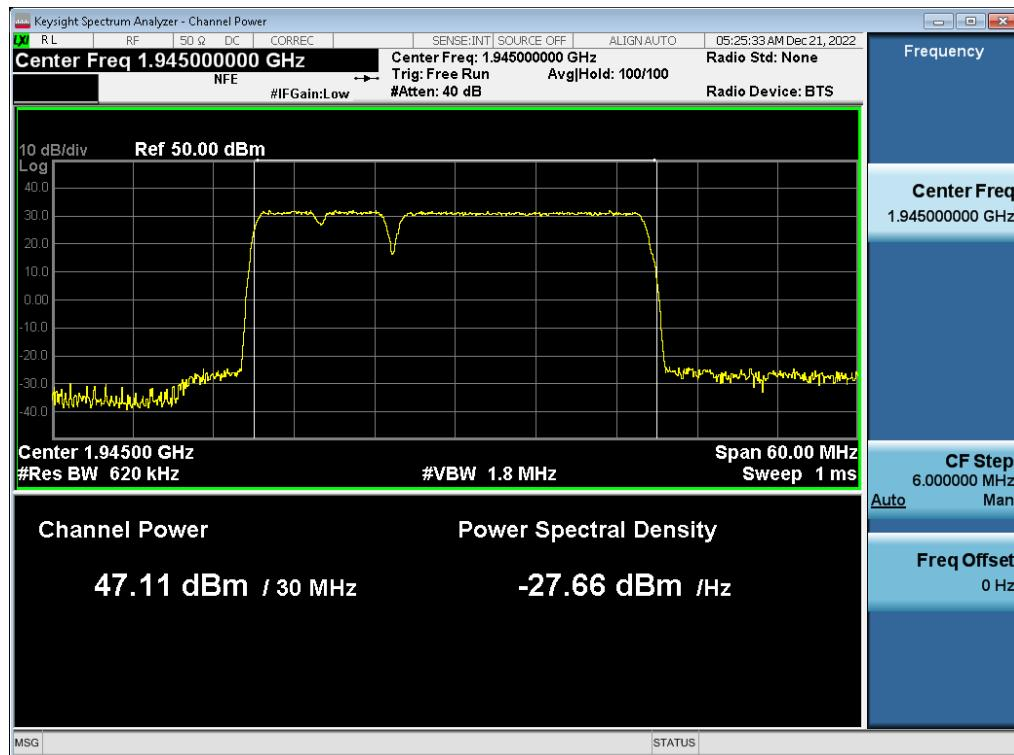
**Antenna 0 / (2 Port) 5G NR n2 5 MHz 1 Carrier + 5G NR n2 5 MHz 1 Carrier + 5G NR n2 5 MHz 1 Carrier [3 Carrier] / 256QAM / Low / Contiguous**
