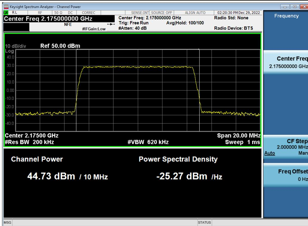
**Antenna 1 / (2 Port) LTE B66 5 MHz 1 Carrier + 5G NR n66 5 MHz 1 Carrier + DSS B66 10 MHz 1 Carrier + DSS B66 20 MHz 1 Carrier [4 Carrier] [1C+3C] / LTE B66 5 MHz 1 Carrier / 64QAM / Low / Non-Contiguous**
