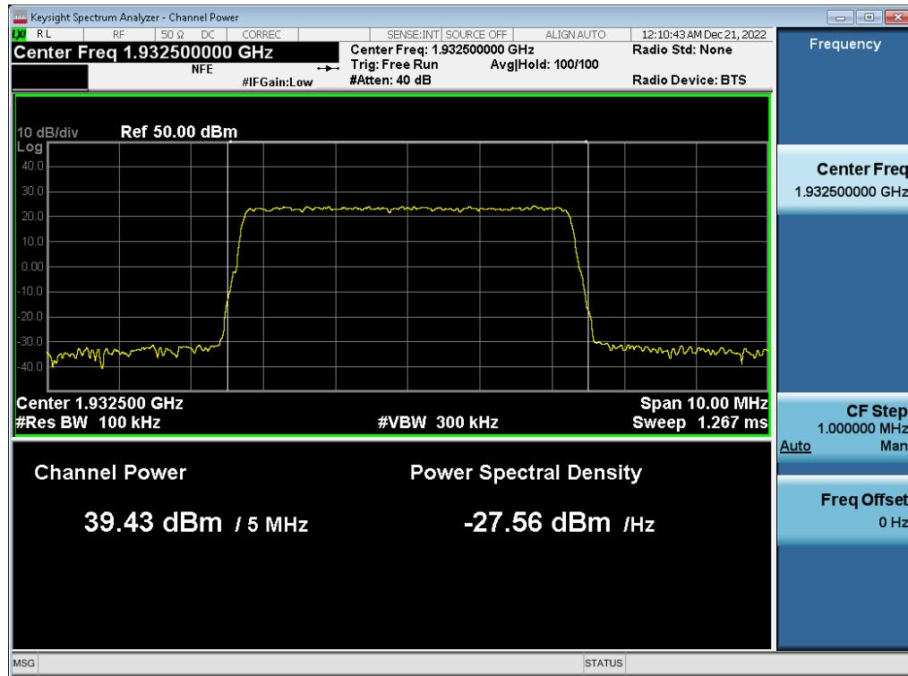
**Antenna 1 / (2 Port) 5G NR n2 5 MHz 1 Carrier + 5G NR n2 5 MHz 1 Carrier + DSS B2 20 MHz 1 Carrier [3 Carrier] [1C+2C] / 5G NR n2 5 MHz 1 Carrier + DSS B2 20 MHz 1 Carrier / 256QAM / High / Non-Contiguous**
