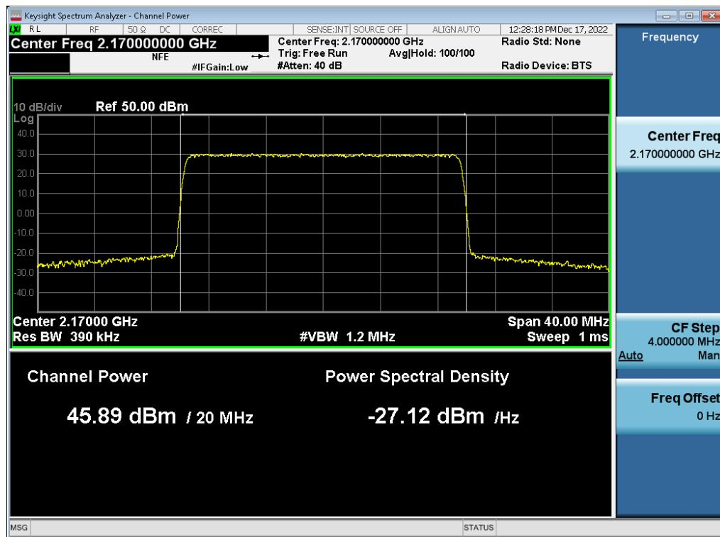
**Antenna 1 / (2 Port) LTE B66 5 MHz 1 Carrier + 5G NR n66 5 MHz 1 Carrier + 5G NR n66 5 MHz 1 Carrier + DSS B66 10 MHz 1 Carrier [4 Carrier] [1C+3C] / LTE B66 5 MHz 1 Carrier / 64QAM / Low / Non-Contiguous**
