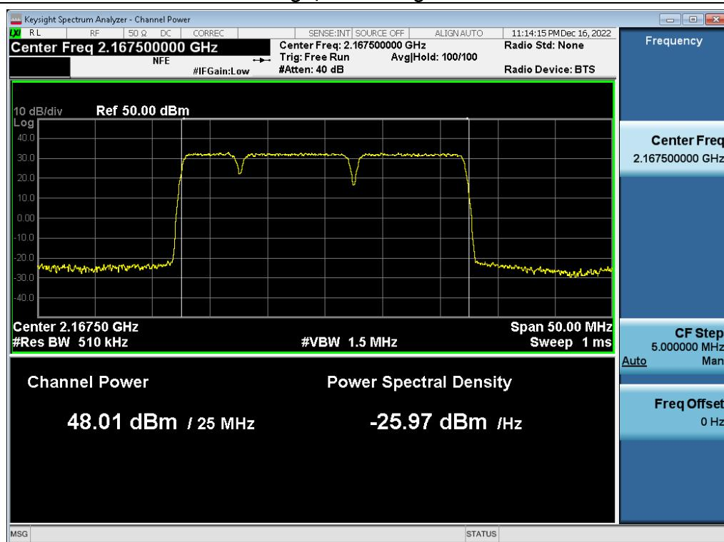
**Antenna 1 / (2 Port) LTE B66 5 MHz 1 Carrier + LTE B66 5 MHz 1 Carrier + DSS B66 10 MHz 1 Carrier + DSS B66 10 MHz 1 Carrier [4 Carrier] [3C+1C] / LTE B66 5 MHz 1 Carrier + LTE B66 5 MHz 1 Carrier + DSS B66 10 MHz 1 Carrier / 16QAM / Low / Non-Contiguous**
