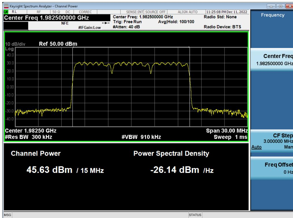
**Antenna 2 / (4 Port) 5G NR n2 5 MHz 1 Carrier + 5G NR n2 5 MHz 1 Carrier + 5G NR n2 20 MHz 1 Carrier [3 Carrier] / 16QAM / Middle / Contiguous**
