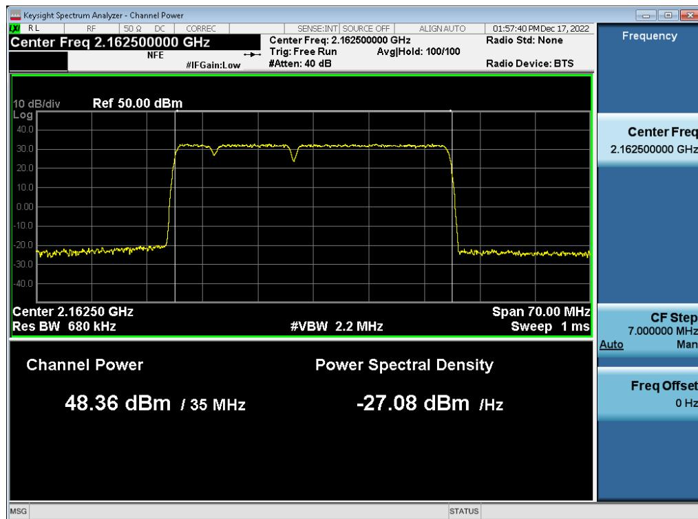
**Antenna 1 / (2 Port) LTE B66 5 MHz 1 Carrier + 5G NR n66 5 MHz 1 Carrier + 5G NR n66 10 MHz 1 Carrier + 5G NR n66 20 MHz 1 Carrier [4 Carrier] [3C+1C] / LTE B66 5 MHz 1 Carrier + 5G NR n66 5 MHz 1 Carrier + 5G NR n66 10 MHz 1 Carrier / QPSK / Low / Non-Contiguous**
