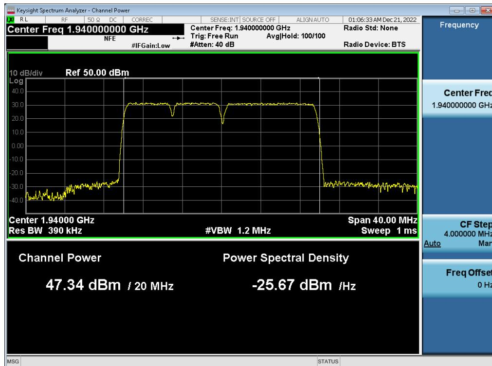
**Antenna 0 / (2 Port) LTE B2 5 MHz 1 Carrier + 5G NR n2 5 MHz 1 Carrier + DSS B2 20 MHz 1 Carrier [3 Carrier] / 256QAM / Low / Contiguous**
