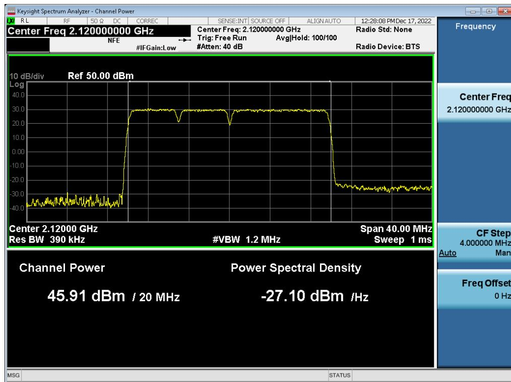
**Antenna 1 / (2 Port) LTE B66 5 MHz 1 Carrier + 5G NR n66 5 MHz 1 Carrier + 5G NR n66 10 MHz 1 Carrier + 5G NR n66 20 MHz 1 Carrier [4 Carrier] [3C+1C] / 5G NR n66 20 MHz 1 Carrier / QPSK / High / Non-Contiguous**
