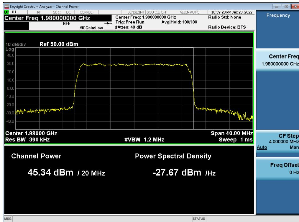
**Antenna 1 / (2 Port) DSS B2 10 MHz 1 Carrier + DSS B2 10 MHz 1 Carrier + DSS B2 10 MHz 1 Carrier [3 Carrier] [1C+2C] / DSS B2 10 MHz 1 Carrier / 64QAM / Low / Non-Contiguous**
