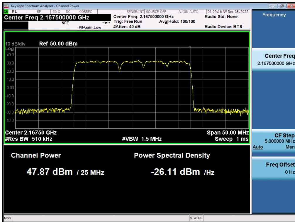
**Antenna 1 / (4 Port) LTE B66 5 MHz 1 Carrier + 5G NR n66 5 MHz 1 Carrier + DSS B66 10 MHz 1 Carrier + DSS B66 20 MHz 1 Carrier [4 Carrier] / 64QAM / Middle / Contiguous**
