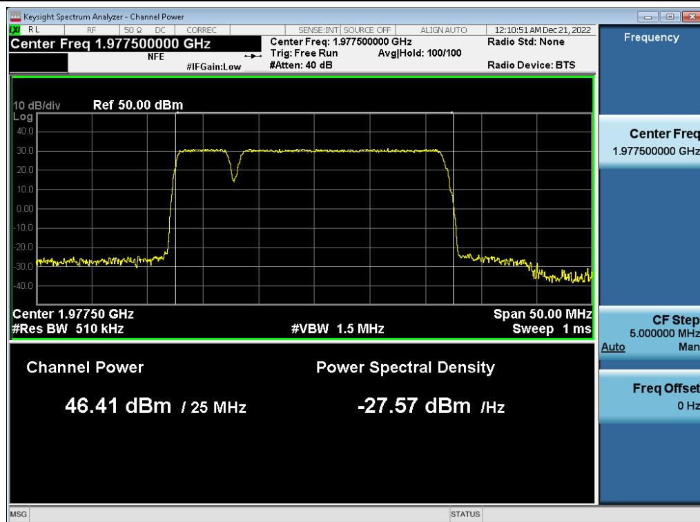
**Antenna 1 / (2 Port) 5G NR n2 5 MHz 1 Carrier + 5G NR n2 5 MHz 1 Carrier + DSS B2 20 MHz 1 Carrier [3 Carrier] [2C+1C] / 5G NR n2 5 MHz 1 Carrier + 5G NR n2 5 MHz 1 Carrier / 16QAM / Low / Non-Contiguous**
