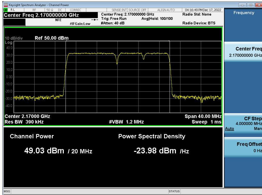
**Antenna 1 / (2 Port) DSS B66 10 MHz 1 Carrier + 5G NR n66 10 MHz 1 Carrier + 5G NR n66 20 MHz 1 Carrier [3 Carrier] / 16QAM / Middle / Contiguous**
