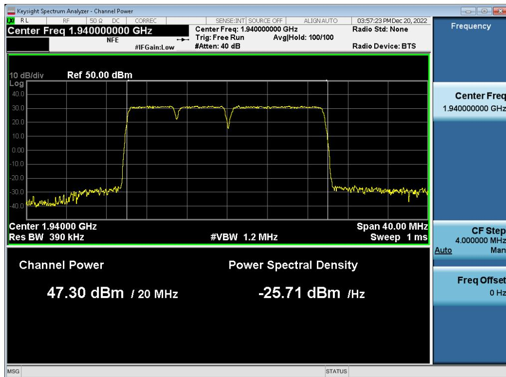
**Antenna 0 / (2 Port) 5G NR n2 5 MHz 1 Carrier + 5G NR n2 5 MHz 1 Carrier + DSS B2 20 MHz 1 Carrier [3 Carrier] / 256QAM / Middle / Contiguous**
