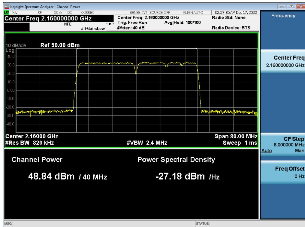
**Antenna 3 / (4 Port) DSS B2 10 MHz 1 Carrier + DSS B2 10 MHz 1 Carrier [2 Carrier] / 256QAM / Middle / Contiguous**
