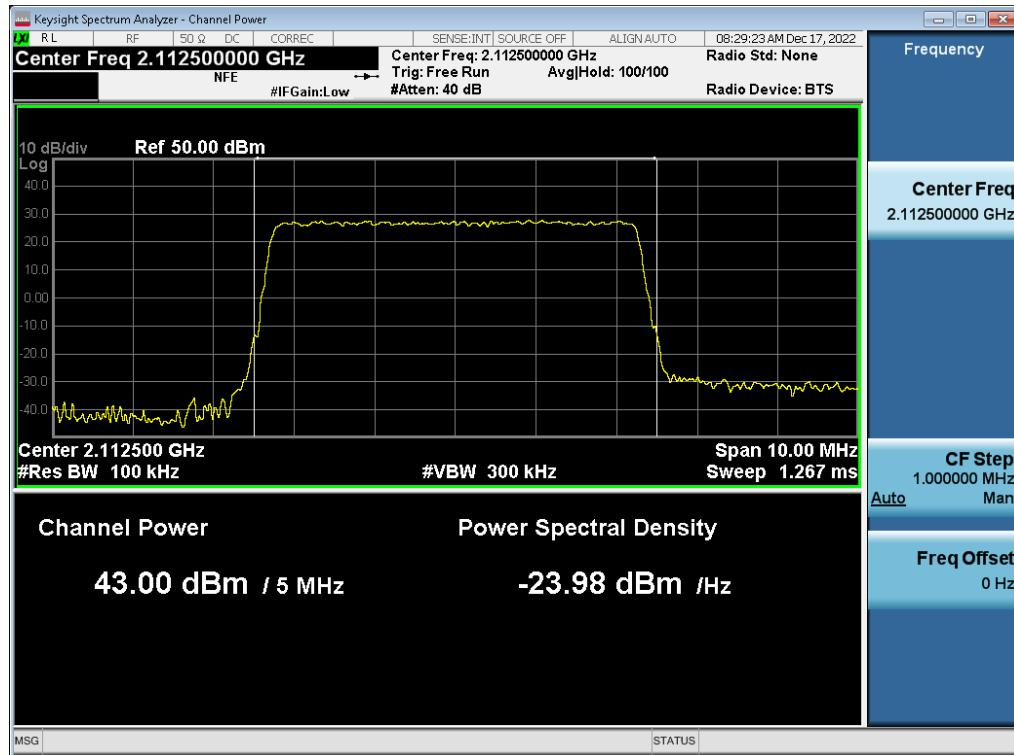
**Antenna 1 / (2 Port) LTE B66 5 MHz 1 Carrier + 5G NR n66 5 MHz 1 Carrier + 5G NR n66 5 MHz 1 Carrier + 5G NR n66 5 MHz 1 Carrier [4 Carrier] [1C+3C] / 5G NR n66 5 MHz 1 Carrier + 5G NR n66 5 MHz 1 Carrier + 5G NR n66 5 MHz 1 Carrier / 256QAM / High / Non-Contiguous**
