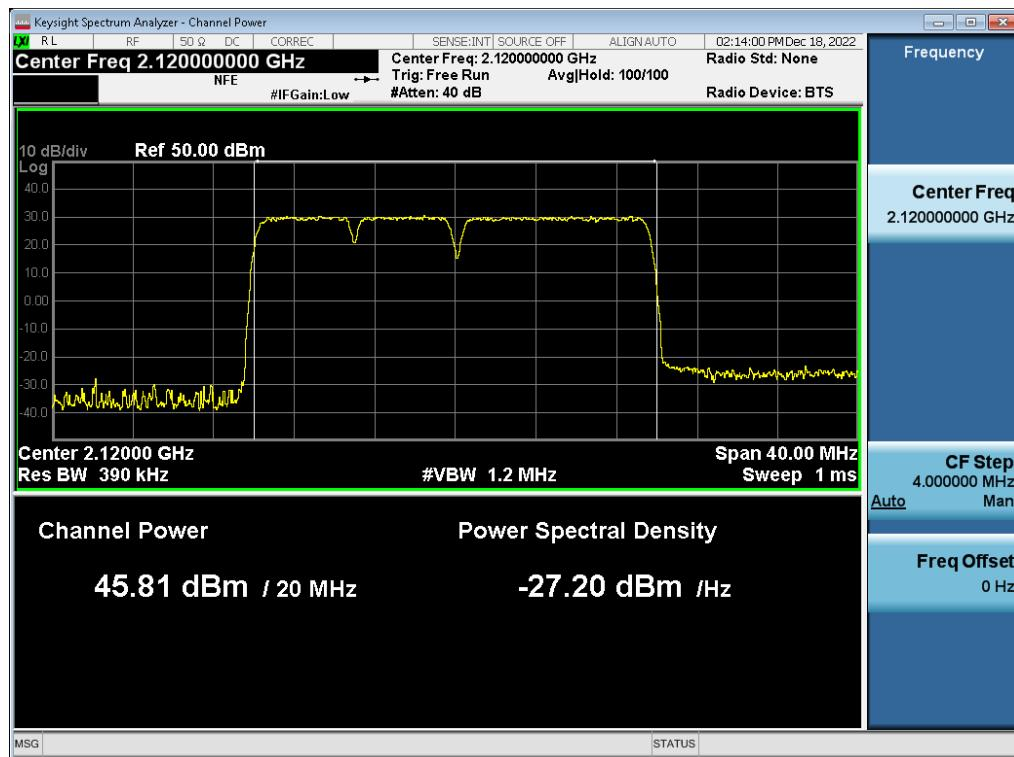
**Antenna 1 / (2 Port) LTE B66 5 MHz 1 Carrier + 5G NR n66 5 MHz 1 Carrier + DSS B66 10 MHz 1 Carrier + DSS B66 20 MHz 1 Carrier [4 Carrier] [3C+1C] / DSS B66 20 MHz 1 Carrier / 256QAM / High / Non-Contiguous**
