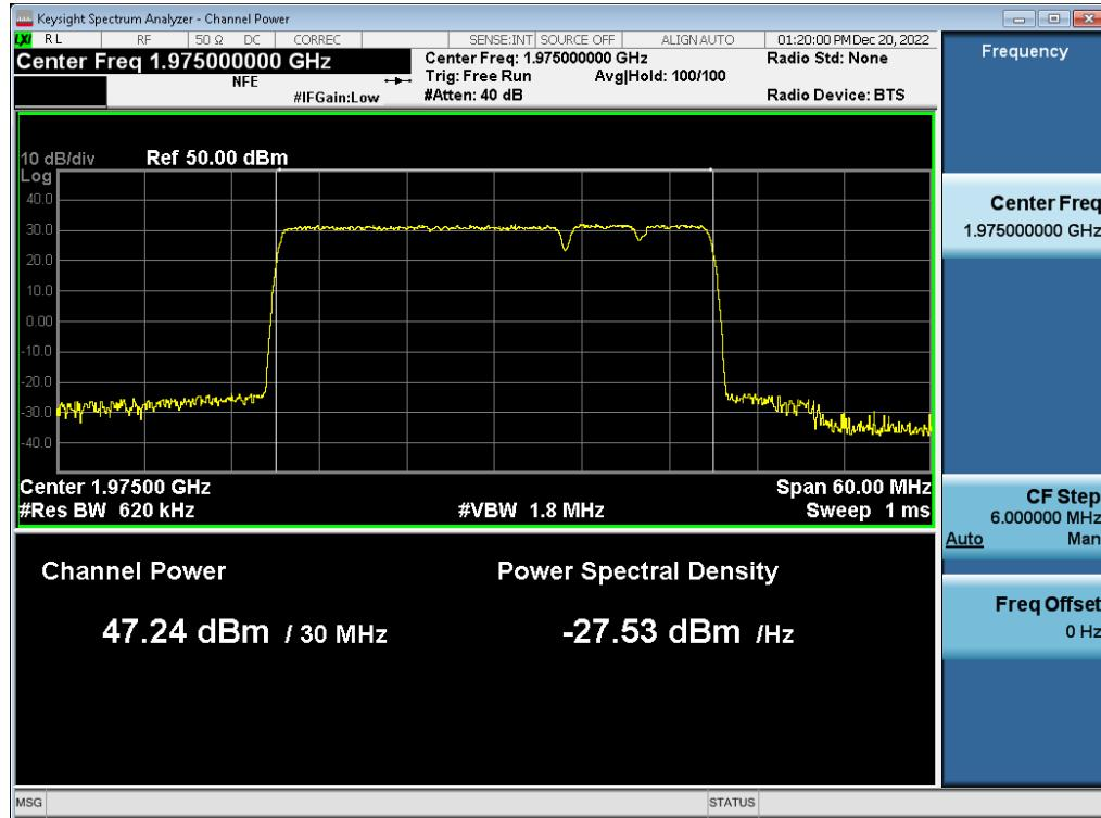
**Antenna 0 / (2 Port) 5G NR n2 5 MHz 1 Carrier + 5G NR n2 5 MHz 1 Carrier + DSS B2 10 MHz 1 Carrier [3 Carrier] / 256QAM / Low / Contiguous**
