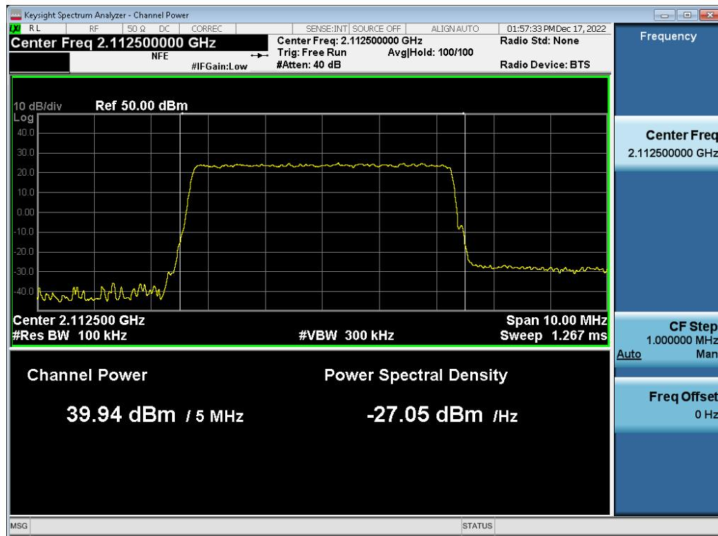
**Antenna 1 / (2 Port) LTE B66 5 MHz 1 Carrier + 5G NR n66 5 MHz 1 Carrier + 5G NR n66 10 MHz 1 Carrier + 5G NR n66 20 MHz 1 Carrier [4 Carrier] [1C+3C] / 5G NR n66 5 MHz 1 Carrier + 5G NR n66 10 MHz 1 Carrier + 5G NR n66 20 MHz 1 Carrier / 256QAM / High / Non-Contiguous**
