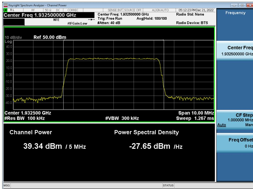
**Antenna 1 / (2 Port) LTE B2 5 MHz 1 Carrier + 5G NR n2 5 MHz 1 Carrier + DSS B2 20 MHz 1 Carrier [3 Carrier] [1C+2C] / 5G NR n2 5 MHz 1 Carrier + DSS B2 20 MHz 1 Carrier / 256QAM / High / Non-Contiguous**
