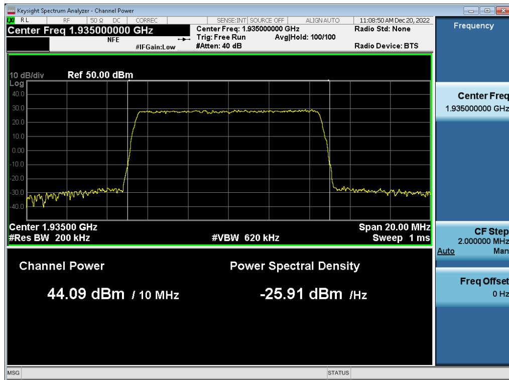
**Antenna 1 / (2 Port) DSS B2 10 MHz 1 Carrier + DSS B2 10 MHz 1 Carrier [2 Carrier] / DSS B2 10 MHz 1 Carrier / 256QAM / High / Non-Contiguous**
