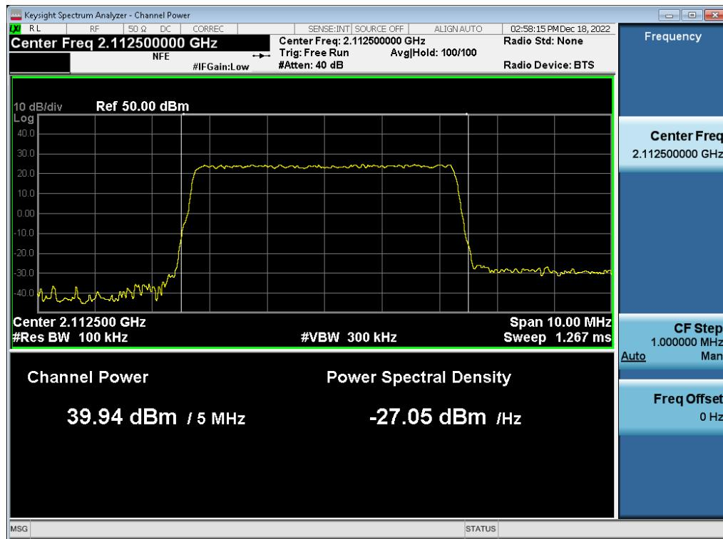
**Antenna 1 / (2 Port) LTE B66 5 MHz 1 Carrier + 5G NR n66 5 MHz 1 Carrier + DSS B66 10 MHz 1 Carrier + DSS B66 20 MHz 1 Carrier [4 Carrier] [1C+3C] / 5G NR n66 5 MHz 1 Carrier + DSS B66 10 MHz 1 Carrier + DSS B66 20 MHz 1 Carrier / 64QAM / High / Non-Contiguous**
