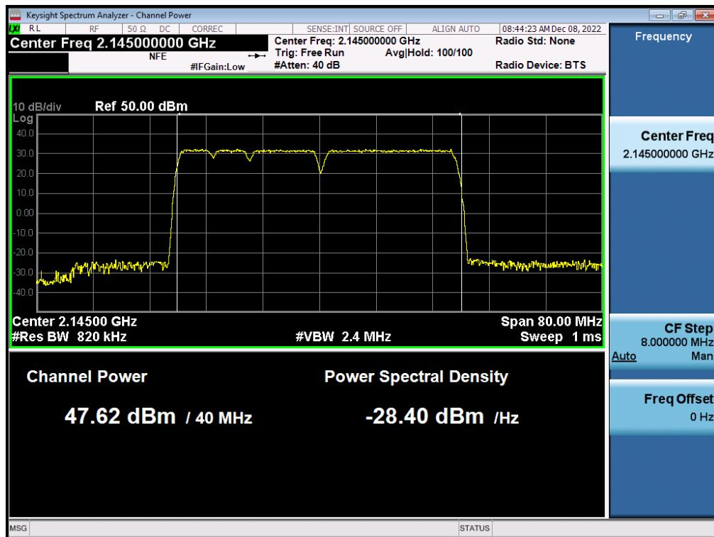
**Antenna 1 / (4 Port) LTE B66 5 MHz 1 Carrier + LTE B66 5 MHz 1 Carrier + DSS B66 10 MHz 1 Carrier + DSS B66 10 MHz 1 Carrier [4 Carrier] / 256QAM / High / Contiguous**
