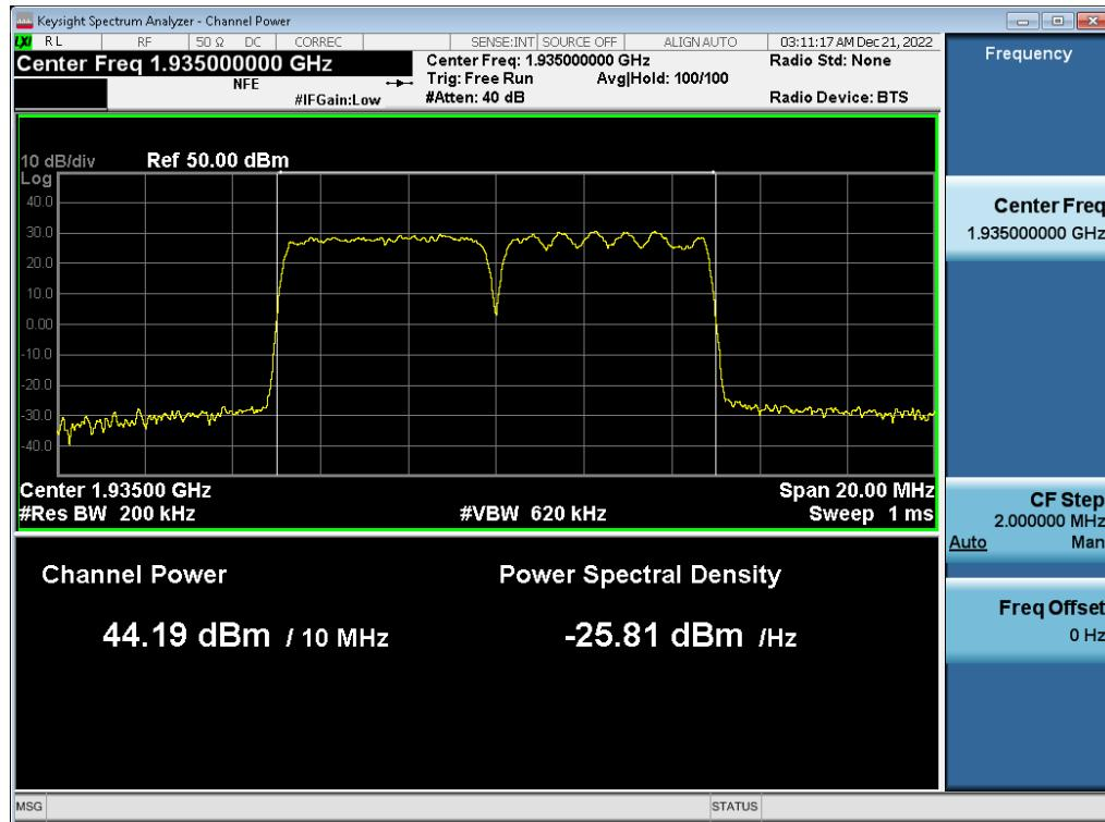
**Antenna 1 / (2 Port) LTE B2 5 MHz 1 Carrier + 5G NR n2 5 MHz 1 Carrier + DSS B2 10 MHz 1 Carrier [3 Carrier] [2C+1C] / DSS B2 10 MHz 1 Carrier / 16QAM / High / Non-Contiguous**
