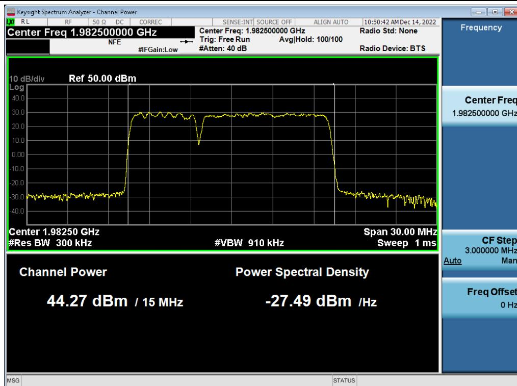
Antenna 2 / (4 Port) LTE B2 5 MHz 1 Carrier + 5G NR n2 5 MHz 1 Carrier + DSS B2 10 MHz 1 Carrier [3 Carrier] [2C+1C] /
