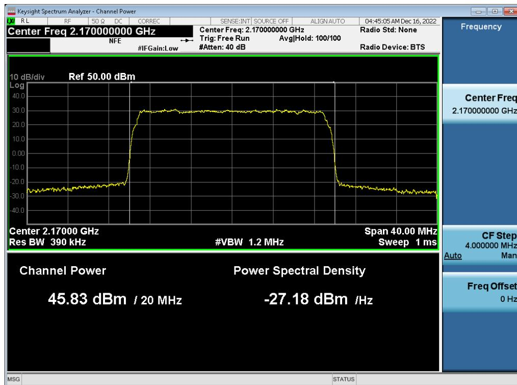
**Antenna 1 / (2 Port) LTE B66 5 MHz 1 Carrier + 5G NR n66 5 MHz 1 Carrier + 5G NR n66 5 MHz 1 Carrier + 5G NR n66 5 MHz 1 Carrier [4 Carrier] [1C+3C] / LTE B66 5 MHz 1 Carrier / 256QAM / Low / Non-Contiguous**
