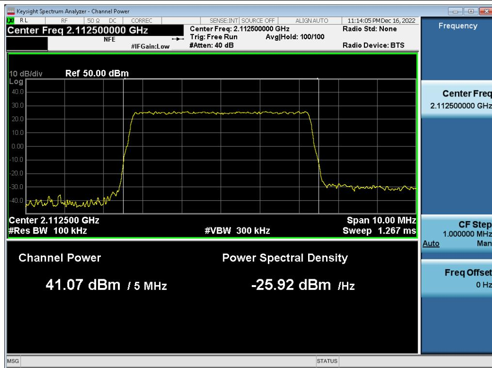
**Antenna 1 / (2 Port) LTE B66 5 MHz 1 Carrier + LTE B66 5 MHz 1 Carrier + DSS B66 10 MHz 1 Carrier + DSS B66 10 MHz 1 Carrier [4 Carrier] [1C+3C] / LTE B66 5 MHz 1 Carrier + DSS B66 10 MHz 1 Carrier + DSS B66 10 MHz 1 Carrier / 256QAM / High / Non-Contiguous**
