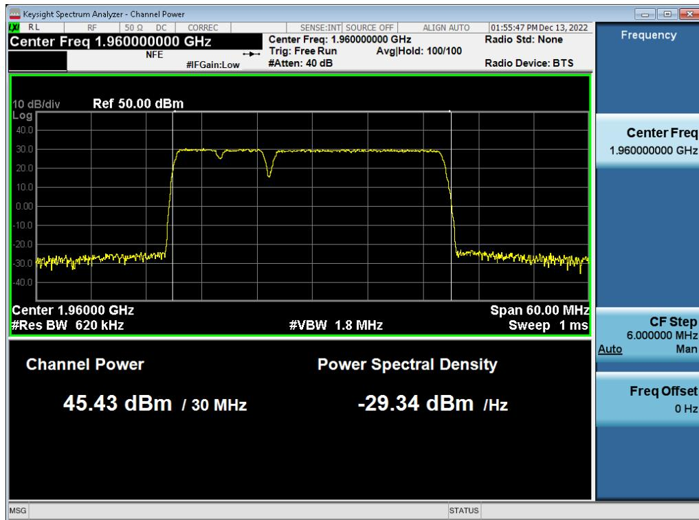
**Antenna 2 / (4 Port) DSS B2 10 MHz 1 Carrier + DSS B2 10 MHz 1 Carrier + DSS B2 10 MHz 1 Carrier [3 Carrier] / 16QAM / Low / Contiguous**
