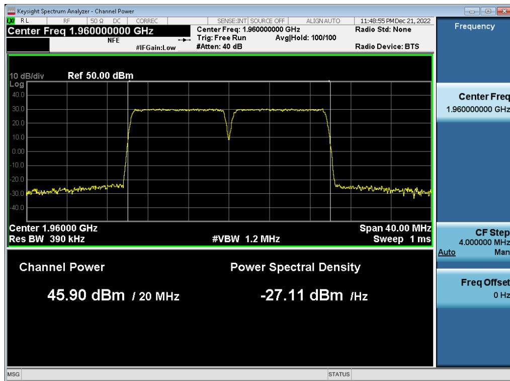
**Antenna 2 / (4 Port) LTE B2 5 MHz 1 Carrier + 5G NR n2 5 MHz 1 Carrier + DSS B2 10 MHz 1 Carrier [3 Carrier] / 256QAM / Low / Contiguous**
