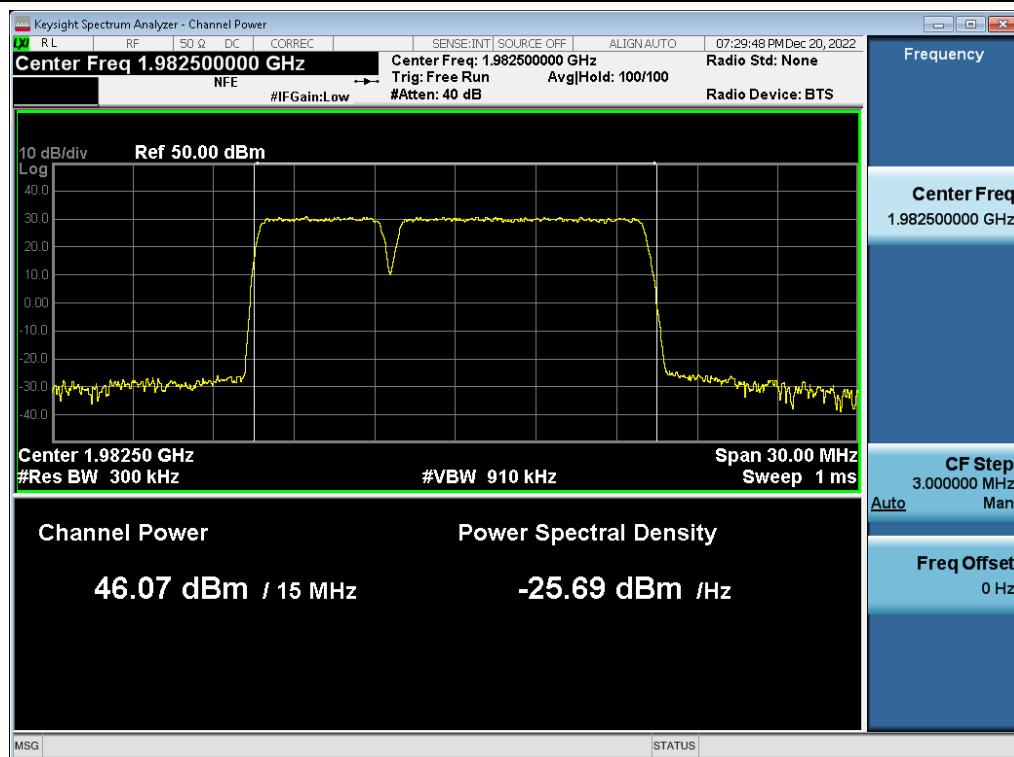
**Antenna 1 / (2 Port) 5G NR n2 5 MHz 1 Carrier + 5G NR n2 5 MHz 1 Carrier + DSS B2 10 MHz 1 Carrier [3 Carrier] [2C+1C] / 5G NR n2 5 MHz 1 Carrier + 5G NR n2 5 MHz 1 Carrier / QPSK / Low / Non-Contiguous**
