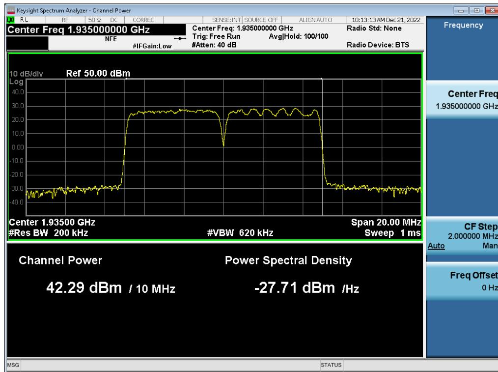
**Antenna 1 / (2 Port) LTE B2 5 MHz 1 Carrier + 5G NR n2 5 MHz 1 Carrier + DSS B2 20 MHz 1 Carrier [3 Carrier] [2C+1C] / DSS B2 20 MHz 1 Carrier / 16QAM / High / Non-Contiguous**
