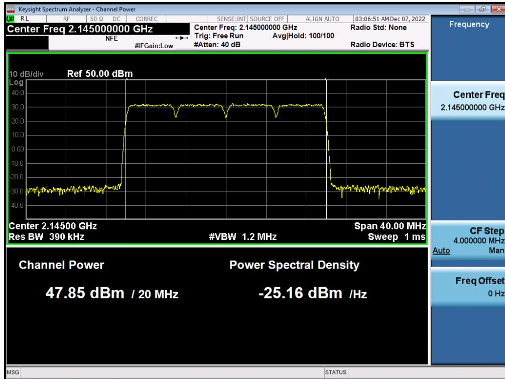
**Antenna 1 / (4 Port) LTE B66 5 MHz 1 Carrier + 5G NR n66 5 MHz 1 Carrier + 5G NR n66 10 MHz 1 Carrier + 5G NR n66 20 MHz 1 Carrier [4 Carrier] / 256QAM / High / Contiguous**
