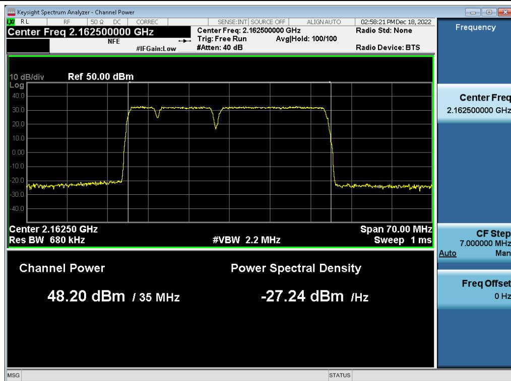
**Antenna 1 / (2 Port) LTE B66 5 MHz 1 Carrier + 5G NR n66 5 MHz 1 Carrier + DSS B66 10 MHz 1 Carrier + DSS B66 20 MHz 1 Carrier [4 Carrier] [3C+1C] / LTE B66 5 MHz 1 Carrier + 5G NR n66 5 MHz 1 Carrier + DSS B66 10 MHz 1 Carrier / 256QAM / Low / Non-Contiguous**
