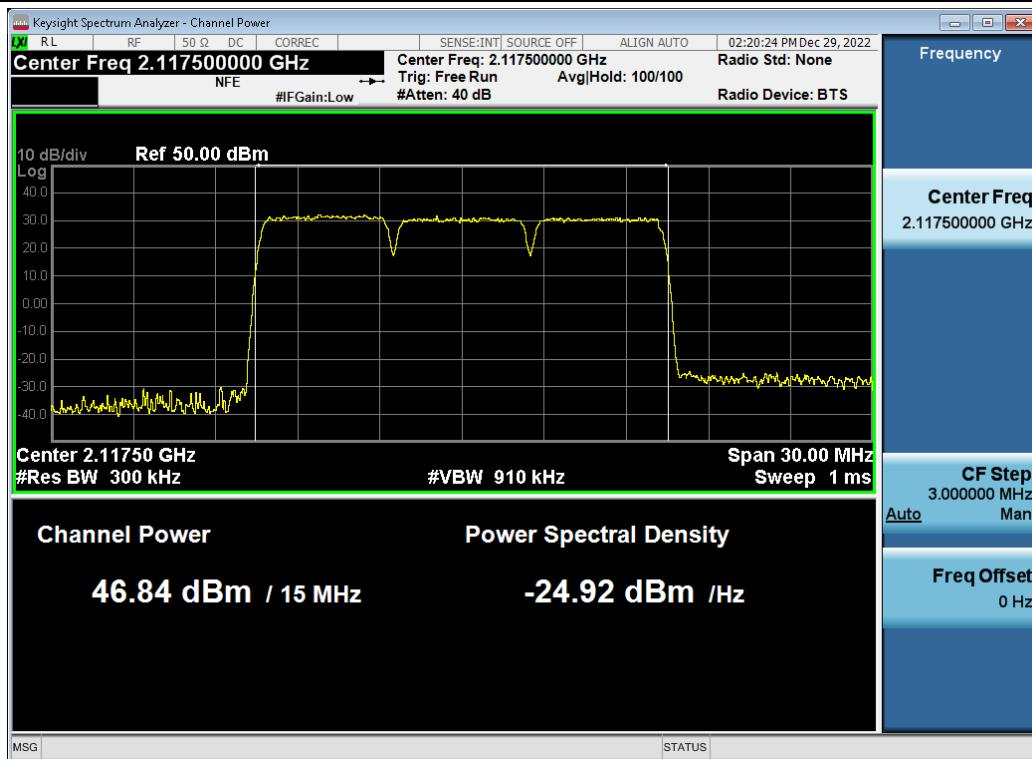
**Antenna 1 / (2 Port) LTE B66 5 MHz 1 Carrier + 5G NR n66 5 MHz 1 Carrier + 5G NR n66 5 MHz 1 Carrier + DSS B66 10 MHz 1 Carrier [4 Carrier] [3C+1C] / DSS B66 10 MHz 1 Carrier / 256QAM / High / Non-Contiguous**
