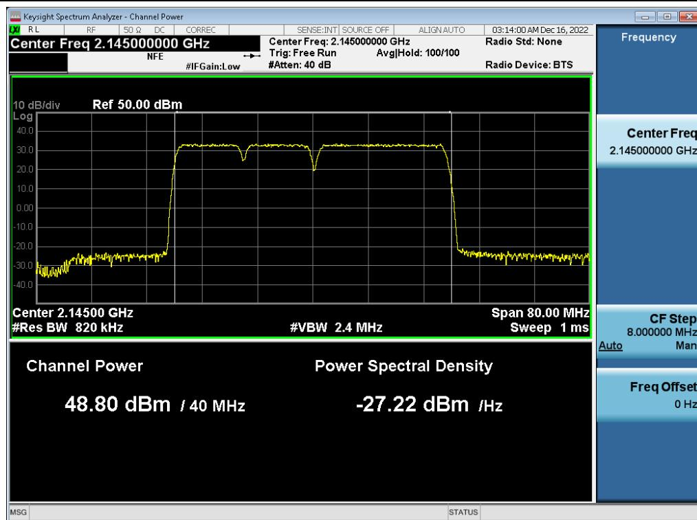
**Antenna 1 / (2 Port) LTE B66 5 MHz 1 Carrier + 5G NR n66 5 MHz 1 Carrier + 5G NR n66 5 MHz 1 Carrier + 5G NR n66 5 MHz 1 Carrier [4 Carrier] / 256QAM / High / Contiguous**
