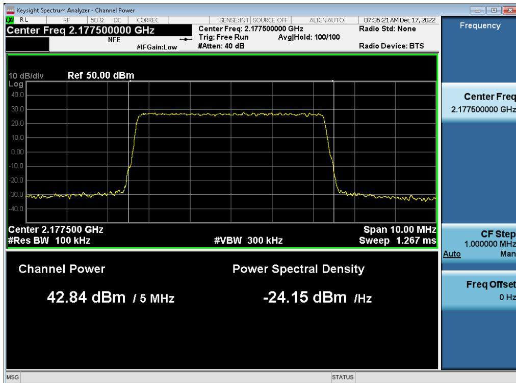
**Antenna 1 / (2 Port) LTE B66 5 MHz 1 Carrier + 5G NR n66 5 MHz 1 Carrier + 5G NR n66 10 MHz 1 Carrier + 5G NR n66 20 MHz 1 Carrier [4 Carrier] [1C+3C] / LTE B66 5 MHz 1 Carrier / 256QAM / Low / Non-Contiguous**
