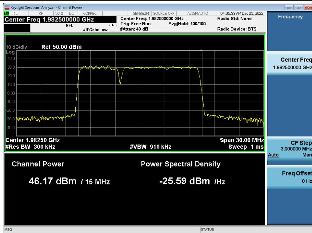
**Antenna 1 / (2 Port) LTE B2 5 MHz 1 Carrier + 5G NR n2 5 MHz 1 Carrier + DSS B2 10 MHz 1 Carrier [3 Carrier] [2C+1C] / LTE B2 5 MHz 1 Carrier + 5G NR n2 5 MHz 1 Carrier / 16QAM / Low / Non-Contiguous**
