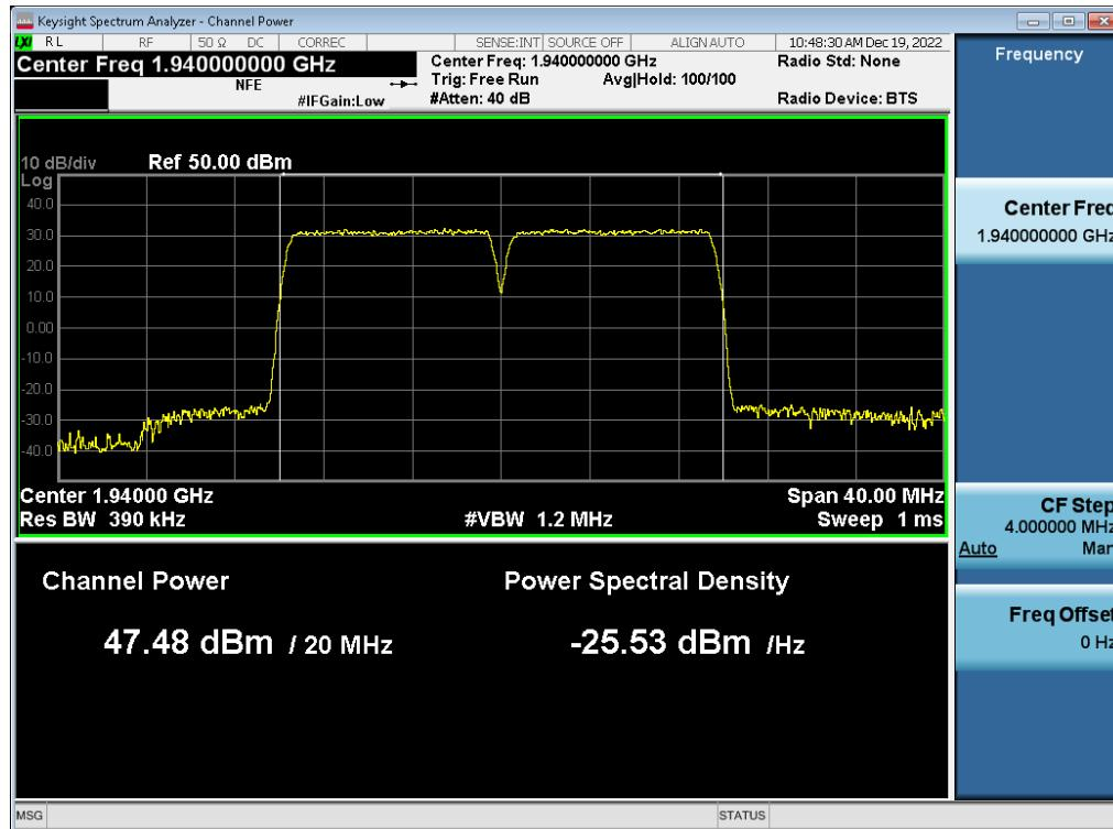
**Antenna 0 / (2 Port) LTE B2 5 MHz 1 Carrier + 5G NR n2 5 MHz 1 Carrier + DSS B2 10 MHz 1 Carrier [3 Carrier] / 256QAM / Low / Contiguous**
