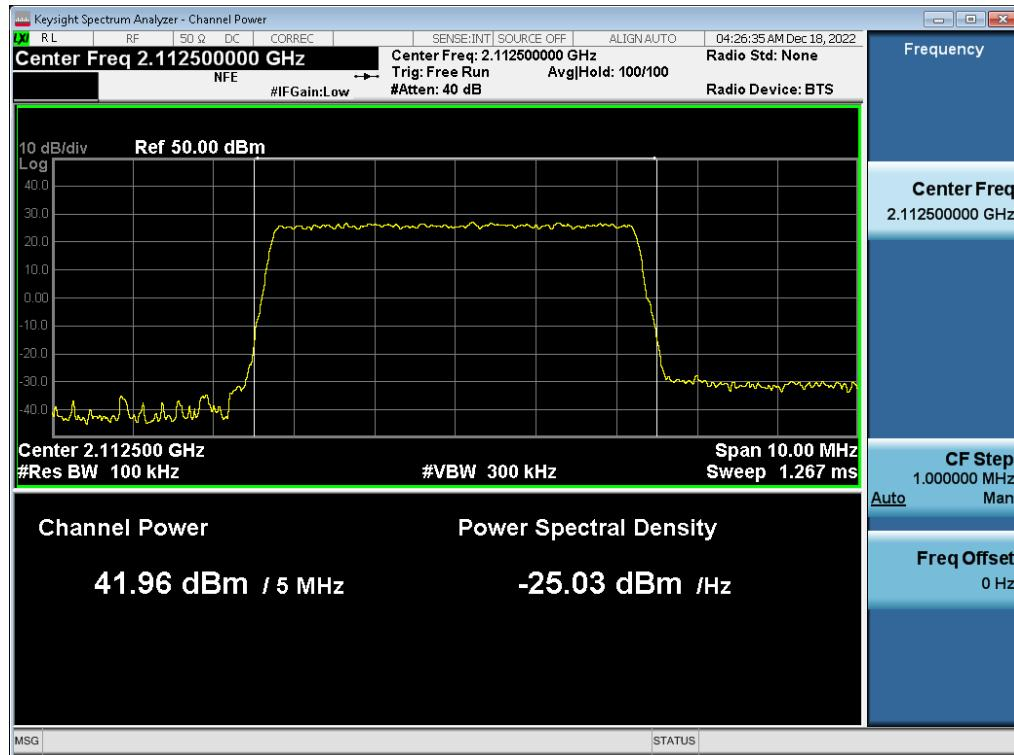
**Antenna 1 / (2 Port) LTE B66 5 MHz 1 Carrier + 5G NR n66 5 MHz 1 Carrier + 5G NR n66 5 MHz 1 Carrier + DSS B66 10 MHz 1 Carrier [4 Carrier] [1C+3C] / 5G NR n66 5 MHz 1 Carrier + 5G NR n66 5 MHz 1 Carrier + DSS B66 10 MHz 1 Carrier / 64QAM / High / Non-Contiguous**
