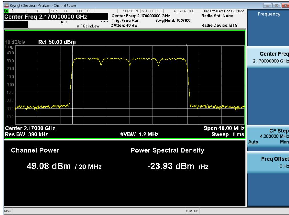
**Antenna 1 / (2 Port) LTE B66 5 MHz 1 Carrier + 5G NR n66 5 MHz 1 Carrier + 5G NR n66 10 MHz 1 Carrier + 5G NR n66 20 MHz 1 Carrier [4 Carrier] / 256QAM / High / Contiguous**
