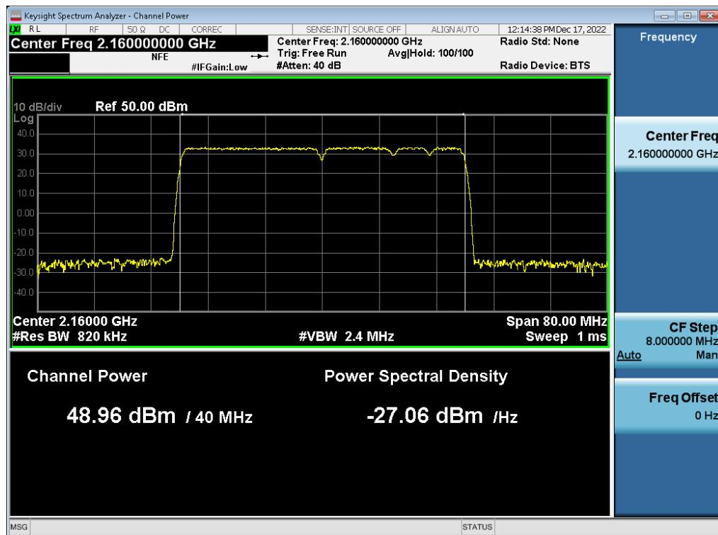
**Antenna 1 / (2 Port) LTE B66 5 MHz 1 Carrier + 5G NR n66 5 MHz 1 Carrier + 5G NR n66 5 MHz 1 Carrier + DSS B66 10 MHz 1 Carrier [4 Carrier] / 256QAM / High / Contiguous**
