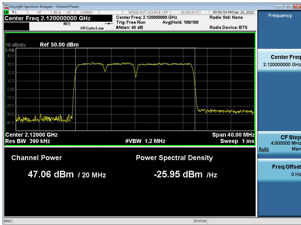
**Antenna 1 / (2 Port) LTE B66 5 MHz 1 Carrier + LTE B66 5 MHz 1 Carrier + DSS B66 10 MHz 1 Carrier + DSS B66 10 MHz 1 Carrier [4 Carrier] [3C+1C] / DSS B66 10 MHz 1 Carrier / 16QAM / High / Non-Contiguous**
