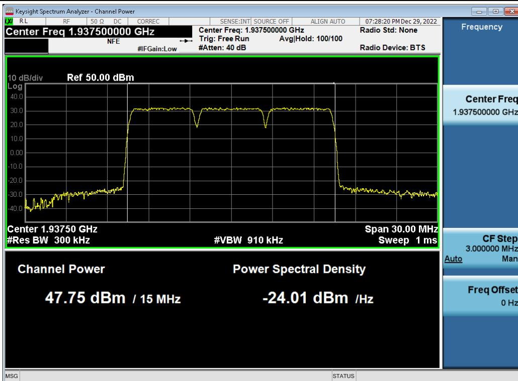
**Antenna 1 / (2 Port) 5G NR n2 5 MHz 1 Carrier + 5G NR n2 5 MHz 1 Carrier + 5G NR n2 20 MHz 1 Carrier [3 Carrier] / 64QAM / High / Contiguous**
