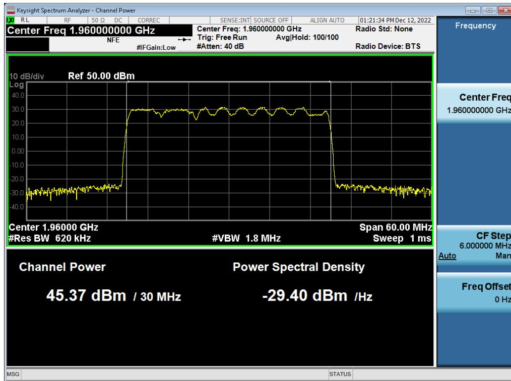
**Antenna 2 / (4 Port) 5G NR n2 5 MHz 1 Carrier + 5G NR n2 5 MHz 1 Carrier + DSS B2 10 MHz 1 Carrier [3 Carrier] / 16QAM / High / Contiguous**
