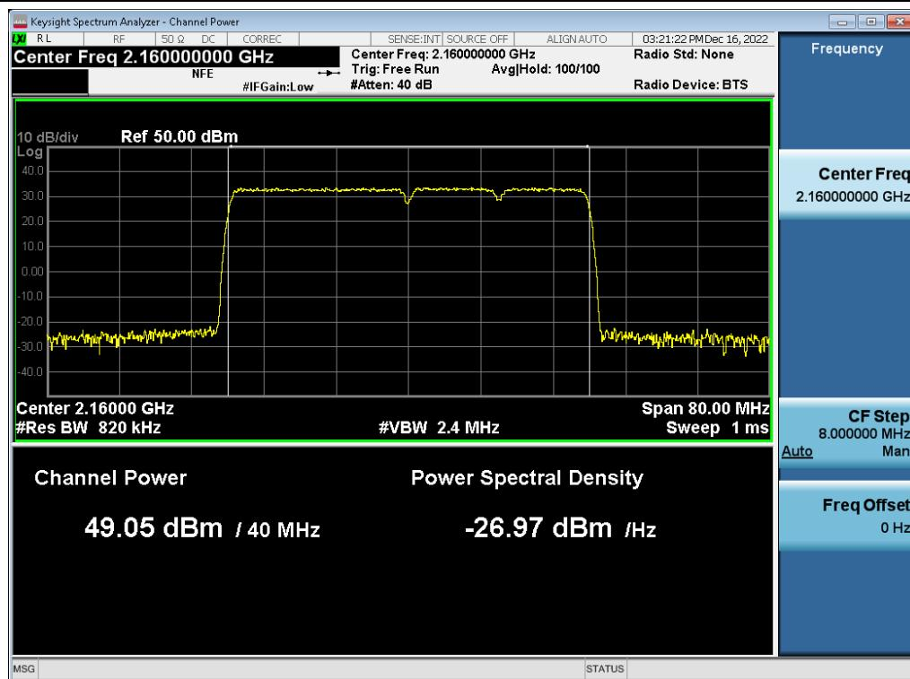
**Antenna 1 / (2 Port) 5G NR n66 5 MHz 1 Carrier + 5G NR n66 5 MHz 1 Carrier + DSS B66 10 MHz 1 Carrier [3 Carrier] / 64QAM / High / Contiguous**
