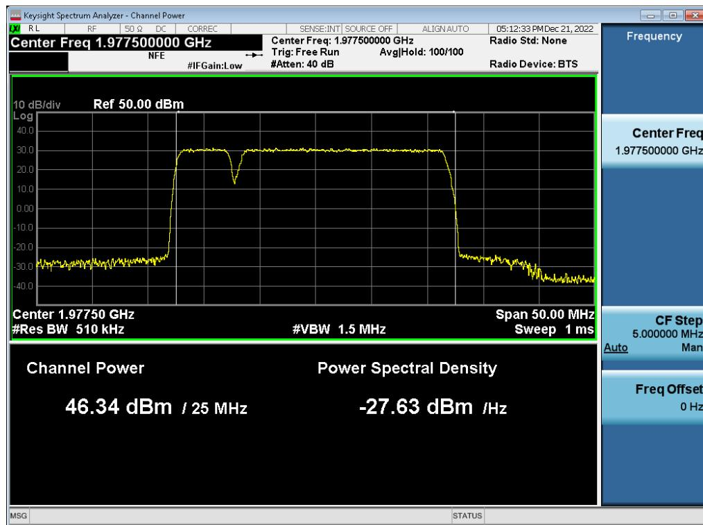
**Antenna 1 / (2 Port) LTE B2 5 MHz 1 Carrier + 5G NR n2 5 MHz 1 Carrier + DSS B2 20 MHz 1 Carrier [3 Carrier] [2C+1C] / LTE B2 5 MHz 1 Carrier + 5G NR n2 5 MHz 1 Carrier / 16QAM / Low / Non-Contiguous**
