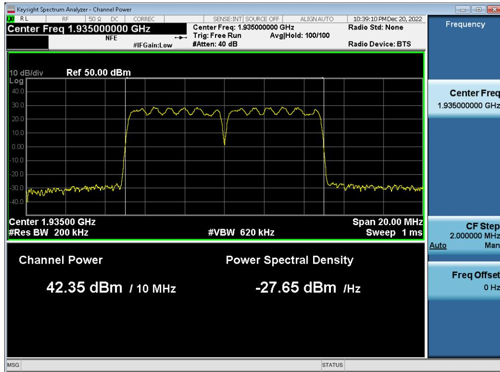
**Antenna 1 / (2 Port) 5G NR n2 5 MHz 1 Carrier + 5G NR n2 5 MHz 1 Carrier + DSS B2 20 MHz 1 Carrier [3 Carrier] [2C+1C] / DSS B2 20 MHz 1 Carrier / 16QAM / High / Non-Contiguous**
