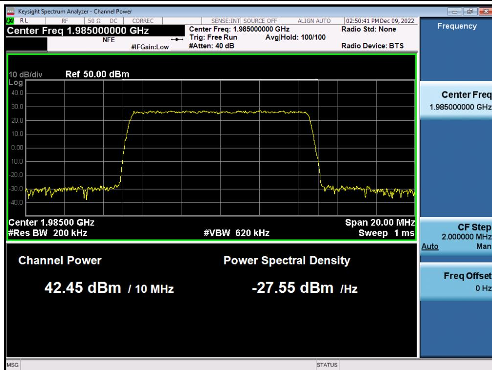
Antenna 2 / (4 Port) LTE B2 5 MHz 1 Carrier + 5G NR n2 5 MHz 1 Carrier + DSS B2 10 MHz 1 Carrier [3 Carrier] [1C+2C] /
