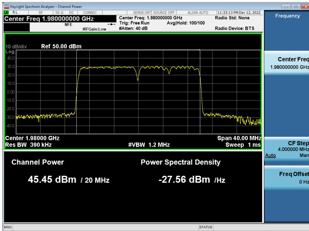
**Antenna 2 / (4 Port) 5G NR n2 5 MHz 1 Carrier + 5G NR n2 5 MHz 1 Carrier + DSS B2 20 MHz 1 Carrier [3 Carrier] / 64QAM / Middle / Contiguous**
