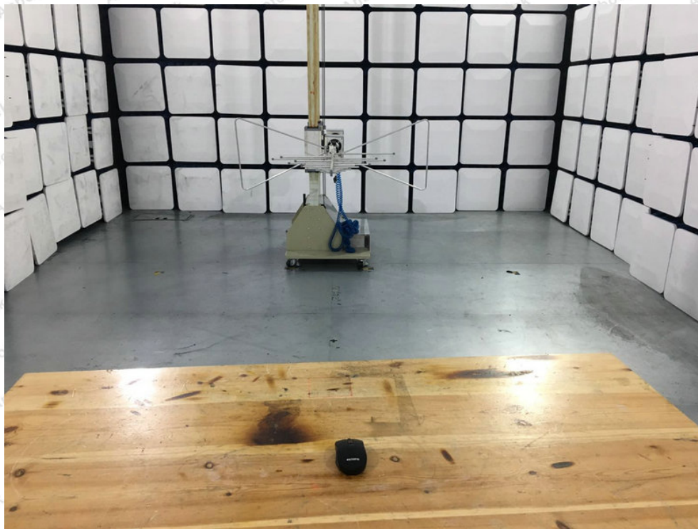
Photo of Radiation Emission Test
