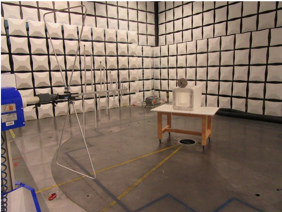
Figure 9 - Test setup for radiated emission on LPR
