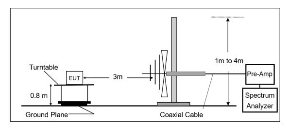
Radiated Emission Test Set-Up, Frequency Above 1GHz.
