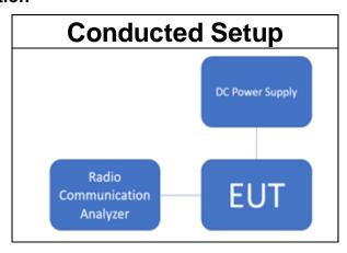
Note: Radio Communication Analyzer is placed in remote side for radiated test.
