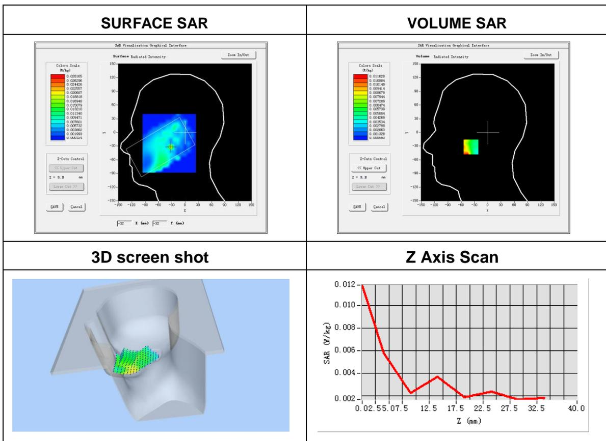
Plot 8: DUT: 5.5inch Smart phone; EUT Model: G25523K
