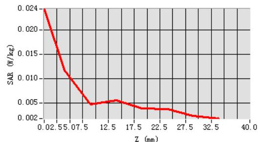
**Plot 2: DUT: 5.5inch Smart phone; EUT Model: G25523K**
