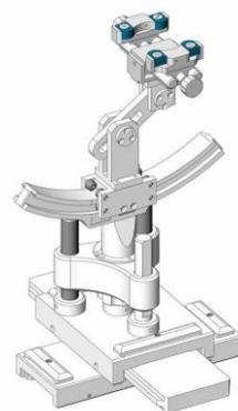
The SAR in the phantom is approximately inversely proportional to the square of the distance between the source and the liquid surface. For a source at 5 mm distance, a positioning uncertainty of  $\pm 0.5$  mm would produce a SAR uncertainty of  $\pm 20$  %. Accurate device positioning is therefore crucial for accurate and repeatable measurements. The positions in which the devices must be measured are defined by the standards.
