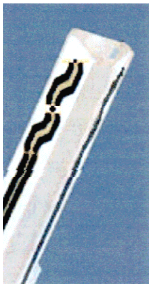
Figure 5. ET3DV6 E-field Probe
