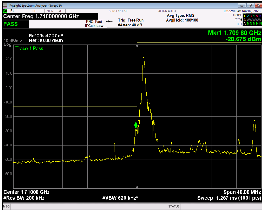
Band4 16QAM BW=20MHz Channel=20050 RB Size=1 Position=#Max
