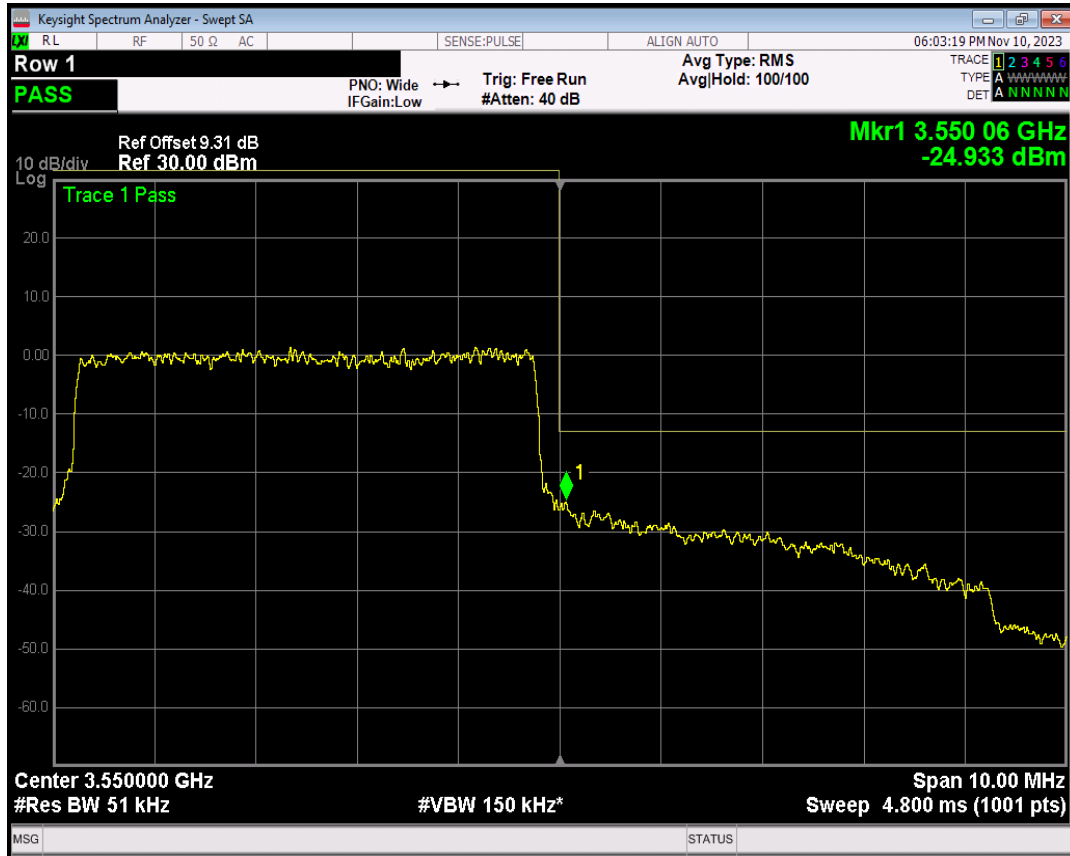
Band42 16QAM BW=5MHz Channel=43065 RB Size=1 Position=#0
