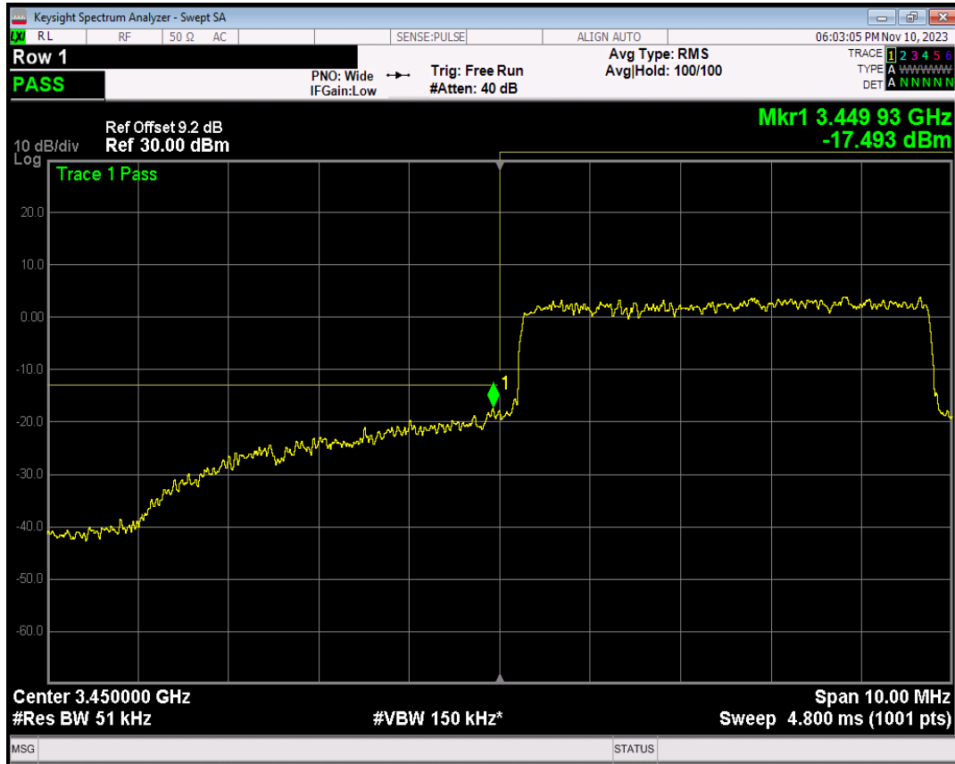
Band42 16QAM BW=5MHz Channel=42115 RB Size=1 Position=#0
