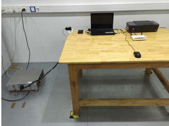
Conducted Emissions Test Setup – Front View
