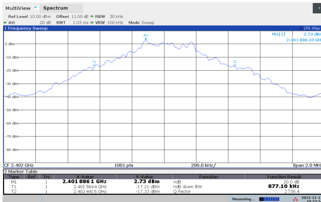
20dB Bandwidth 2402 MHz, GFSK
