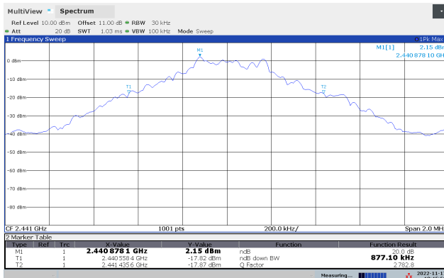
20dB Bandwidth 2441 MHz, GFSK
