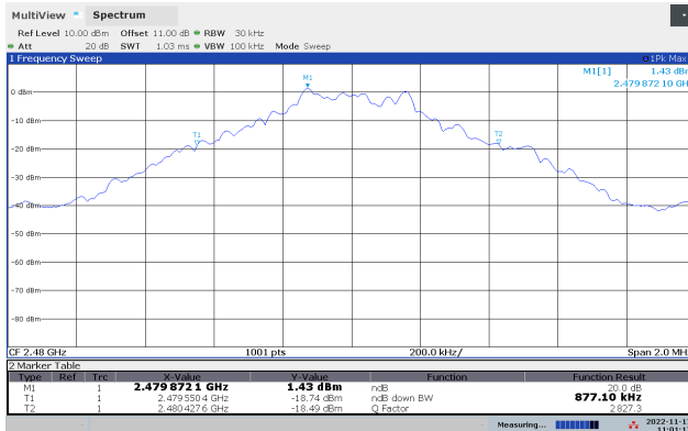
20dB Bandwidth 2480 MHz, GFSK
