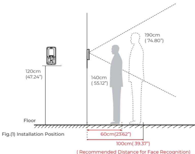
Suggested installation height (the distance between the lens and the ground is 1.2m( 47.24" ), as the recognizable body height range, 0.6m( 23.62" ) distance away from the device, is 1.4-1.6m ( 55.12-63.00" ); the recognizable body height range, 1.0m( 39.37" ) distance away from the device, is 1.6-1.9m(63.00-74.80" ). (There are some deviations) .
