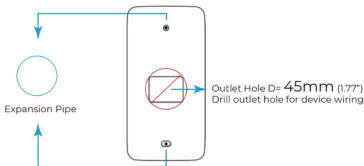
2. Please punch out the tail lines from the outlet hole before installing the mounting bracket and use the screws to fix the mounting bracket on the wall. Use the screwdriver to tighten the screw follow the direction indicated, to complete the installation.
