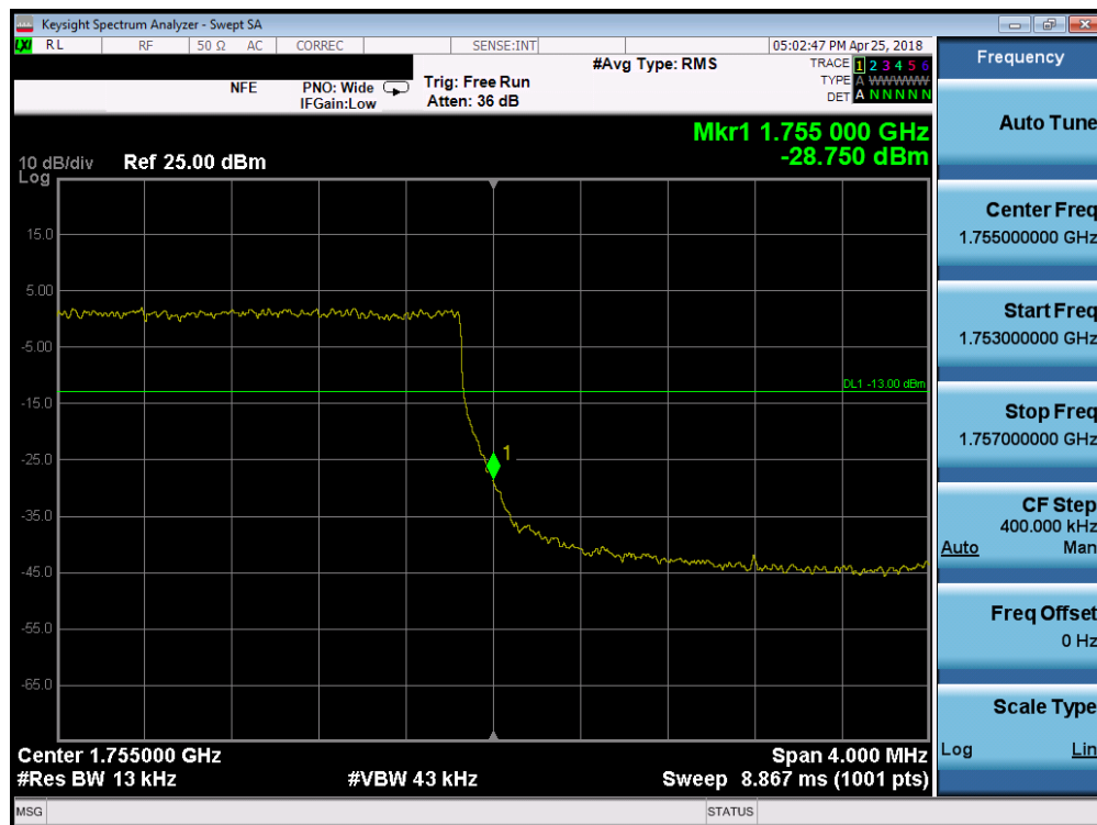
Plot 7-188. Upper Band Edge Plot (Band 4 - 3.0MHz QPSK - Full RB Configuration)
