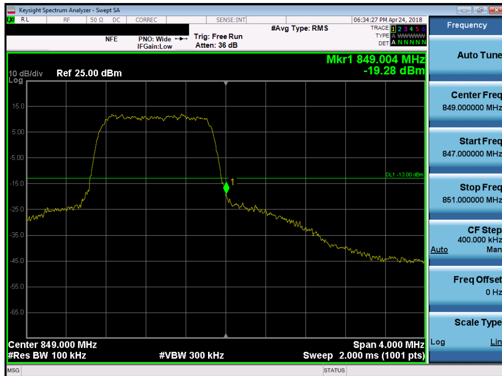
Plot 7-173. Upper Band Edge Plot (Band 5 - 1.4MHz QPSK - Full RB Configuration)
