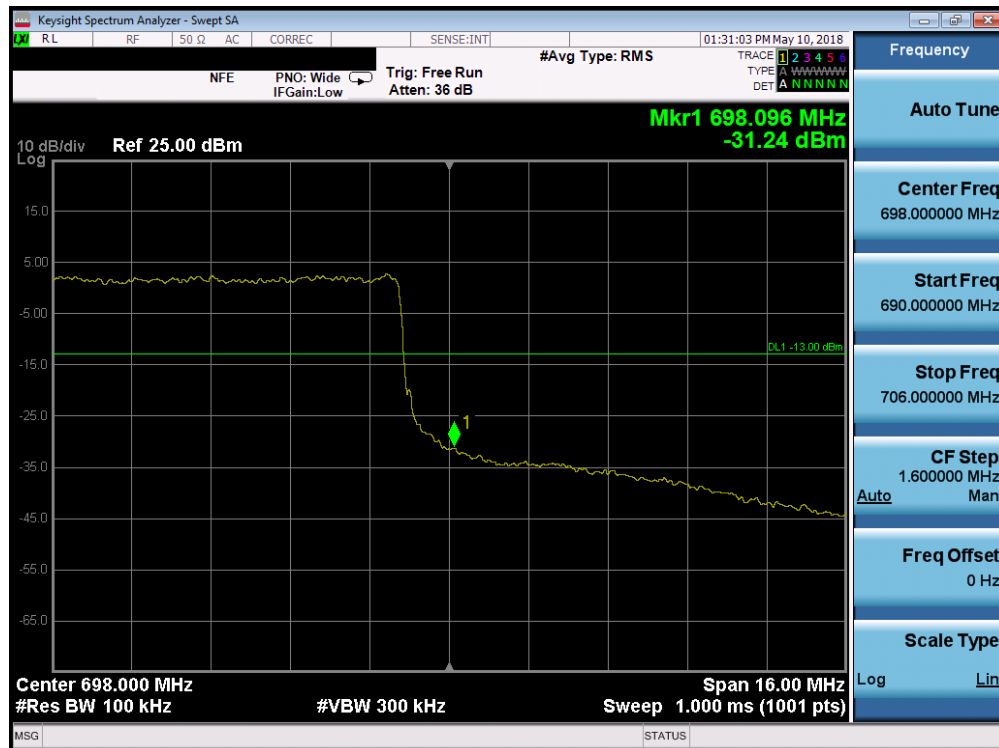
Plot 7-155. Upper Band Edge Plot (Band 71 - 20.0MHz QPSK - Full RB Configuration)
