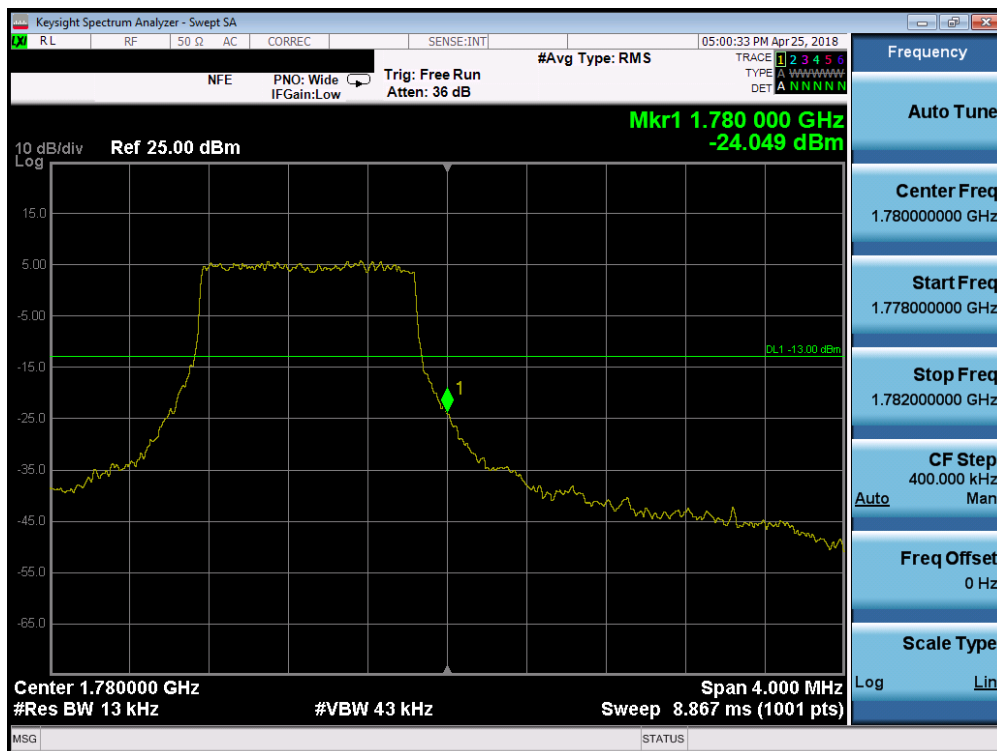
Plot 7-184. Upper Band Edge Plot (Band 66 - 1.4MHz QPSK - Full RB Configuration)
