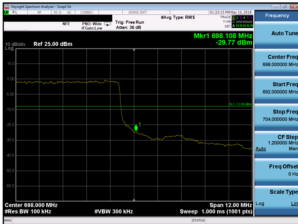
Plot 7-153. Upper Band Edge Plot (Band 71 - 15.0MHz QPSK - Full RB Configuration)
