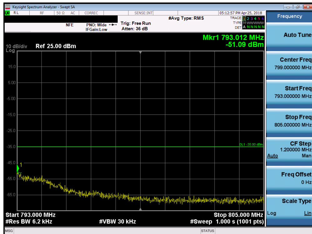
Plot 7-167. Upper Emission Mask Plot (Band 13 - 5.0MHz QPSK - Full RB Configuration)
