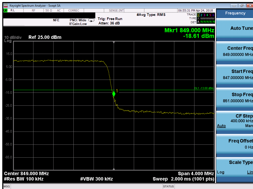
Plot 7-175. Upper Band Edge Plot (Band 5 - 3.0MHz QPSK - Full RB Configuration)
