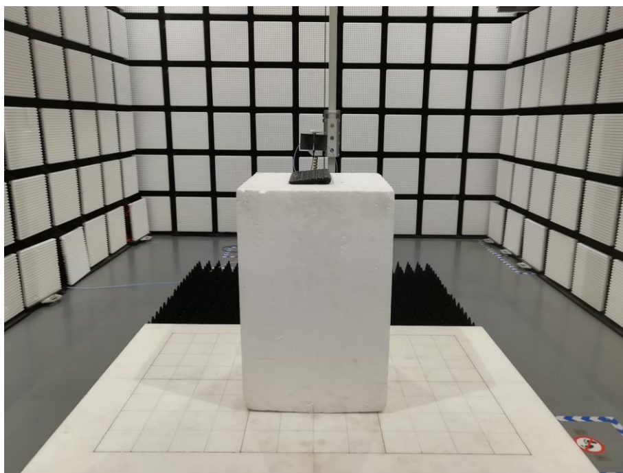
Fig. 3 Radiated emission setup photo(Above 1GHz)
