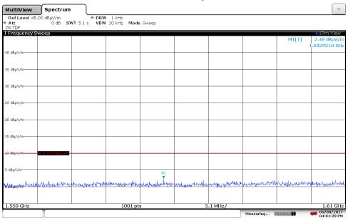
6.5.3.2 Vertical Measurement Polarity 1559 to 1610 MHz
