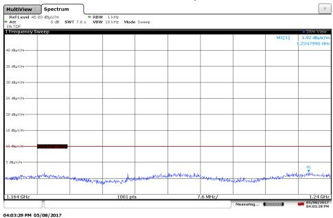
6.5.2.2 Vertical Measurement Polarity 1164 to 1240 MHz
