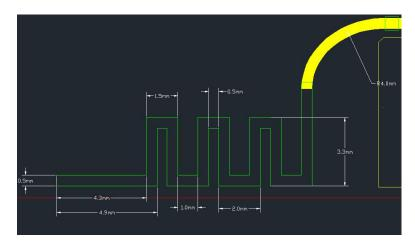
Antenna dimensions as blow picture show (unit: mm): the material is FR4 and the thickness is 1.6mm of PCB.
