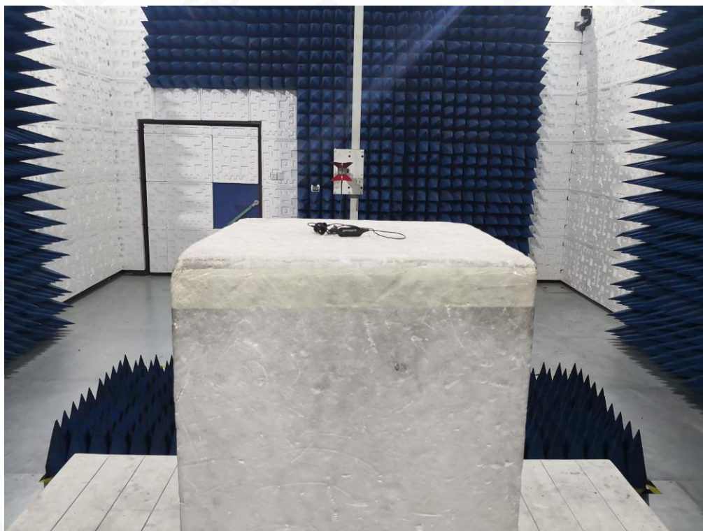
RADIATED EMISSION TEST SETUP ABOVE 1GHZ
