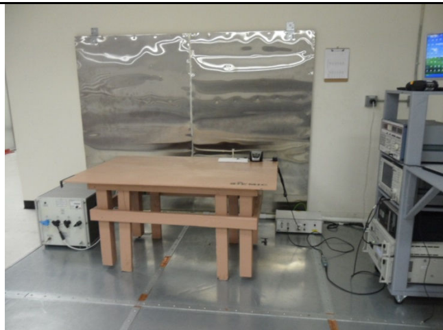
Conducted Emission Test setup - Front
