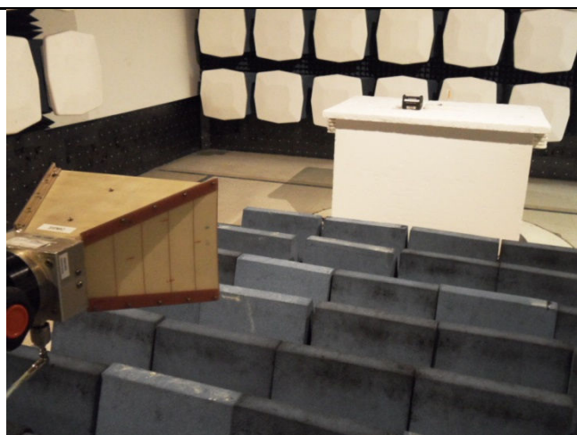
Radiated Emission Test Setup (>1GHz) - Front
