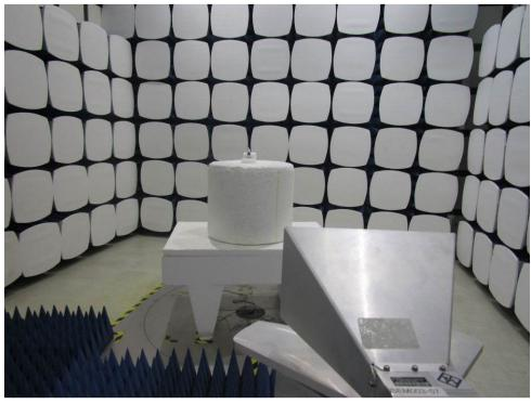
1.2 Radiated Spurious Emissions Test Setup
