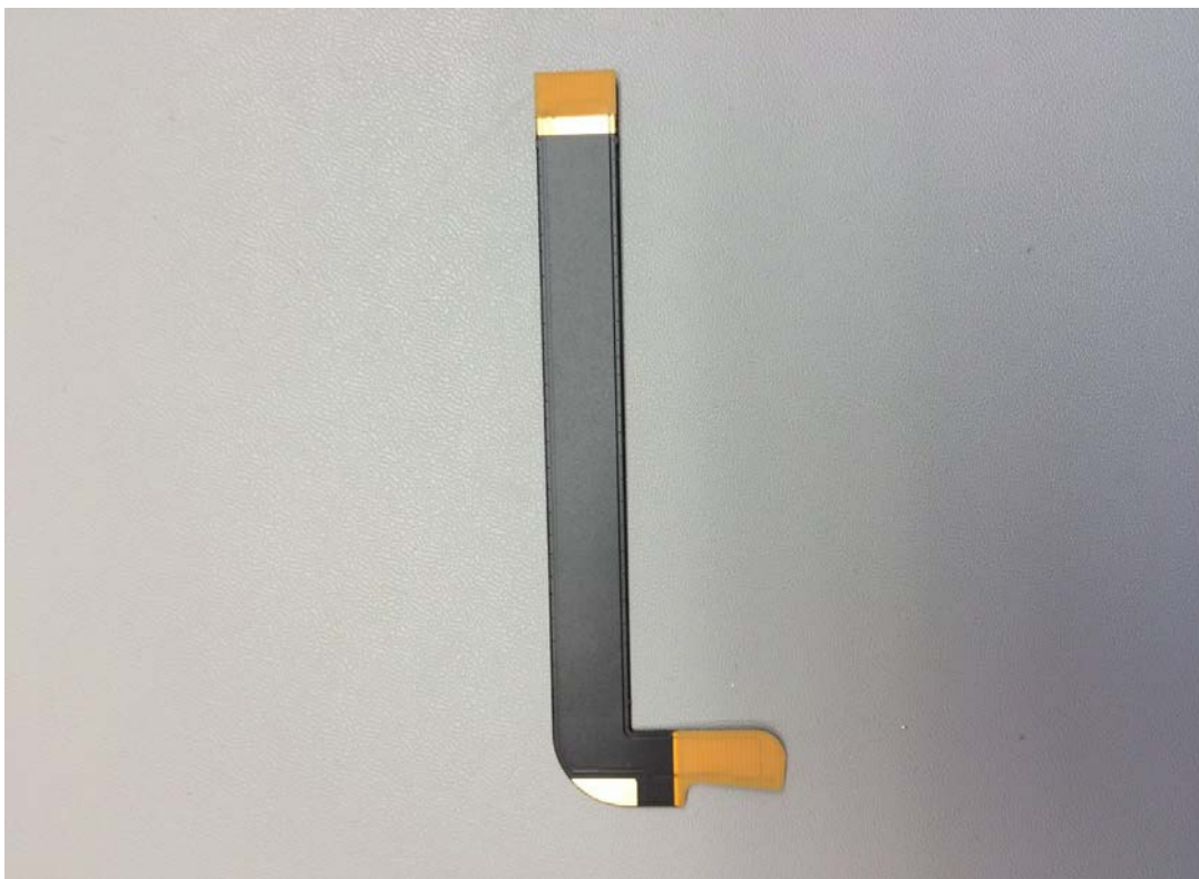
MS2 battery connector flex (front)
