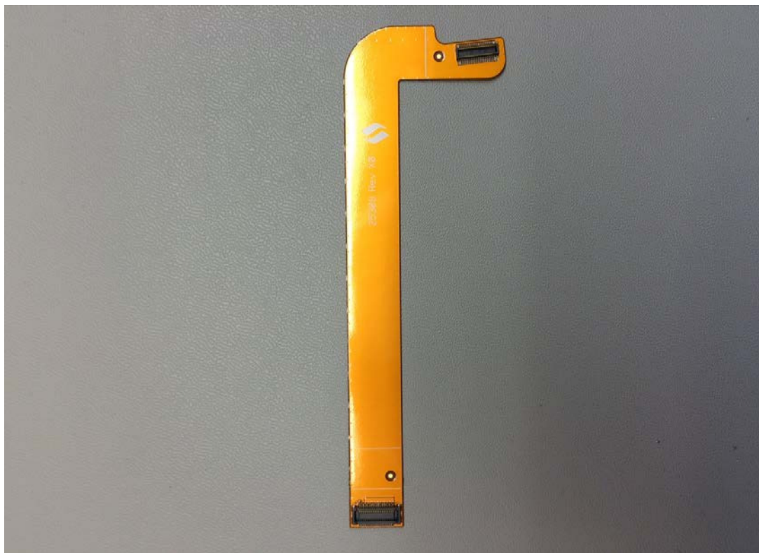
MS2 battery connector flex (back)
