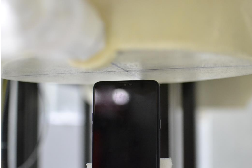
SAR Test Setup Photo 7 – Top at 1.0 cm
