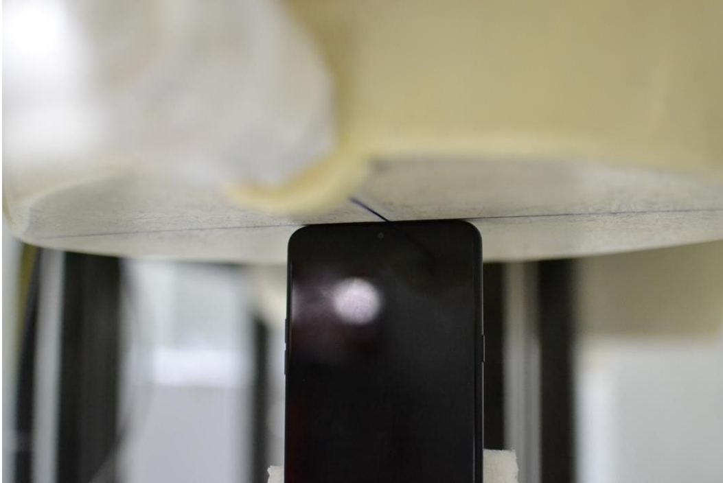
SAR Test Setup Photo 13 – Top at 0.0 cm
