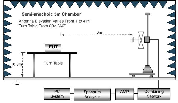
(C) Radiated Emission Test-Up Frequency Above 1GHz
