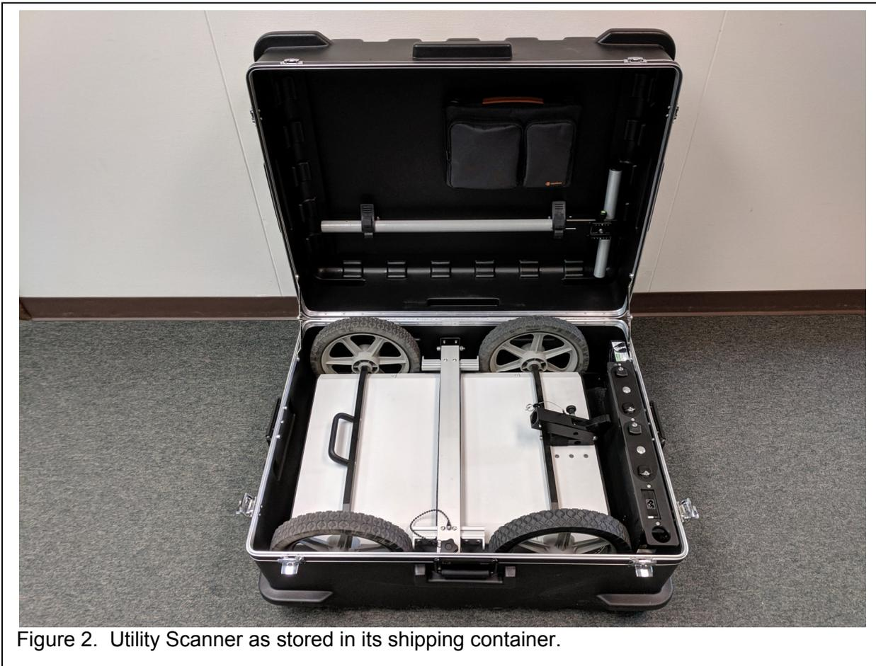
Figure 2. Utility Scanner as stored in its shipping container.
