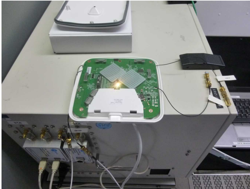
Photo 5 client setup detailed
