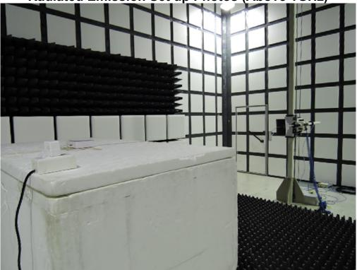
Radiated Emission Set up Photos (Front View)
