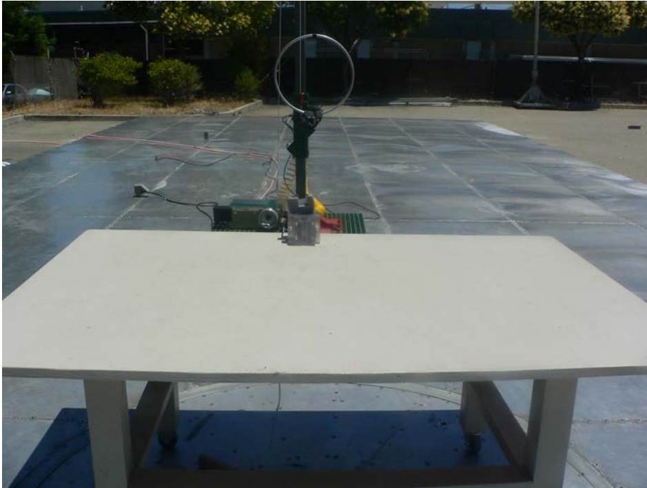
Radiated Emission – Front View (Low Frequency)
