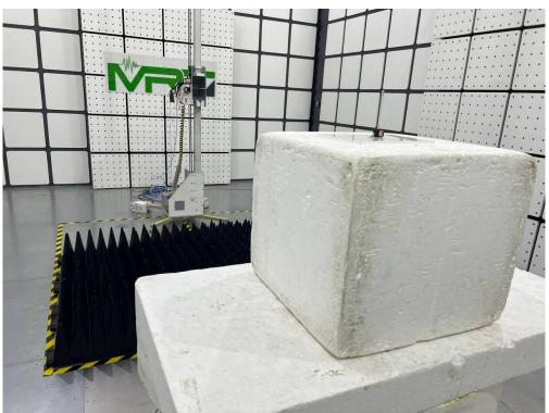
Description: Radiated Emission Test Setup for 1GHz ~ 4GHz
