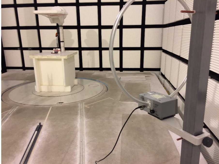
Photo 7: RSE set-up (<30MHz)
