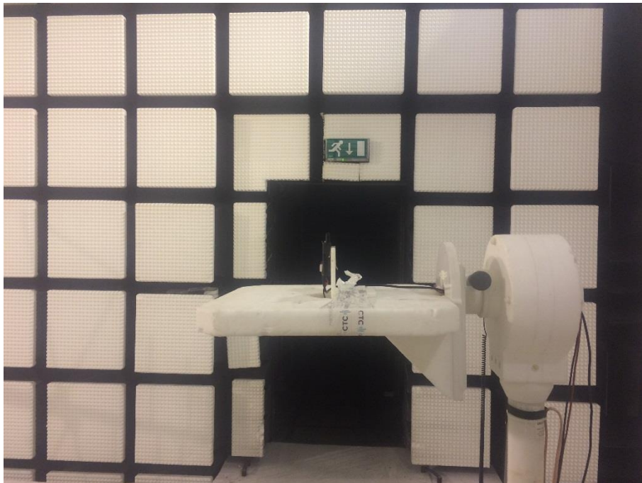
Photo 2: RSE set-up (>1GHz)
