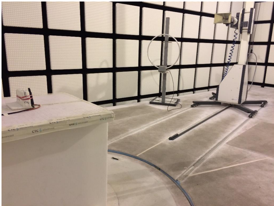
Photo 6: RSE set-up (<30MHz)
