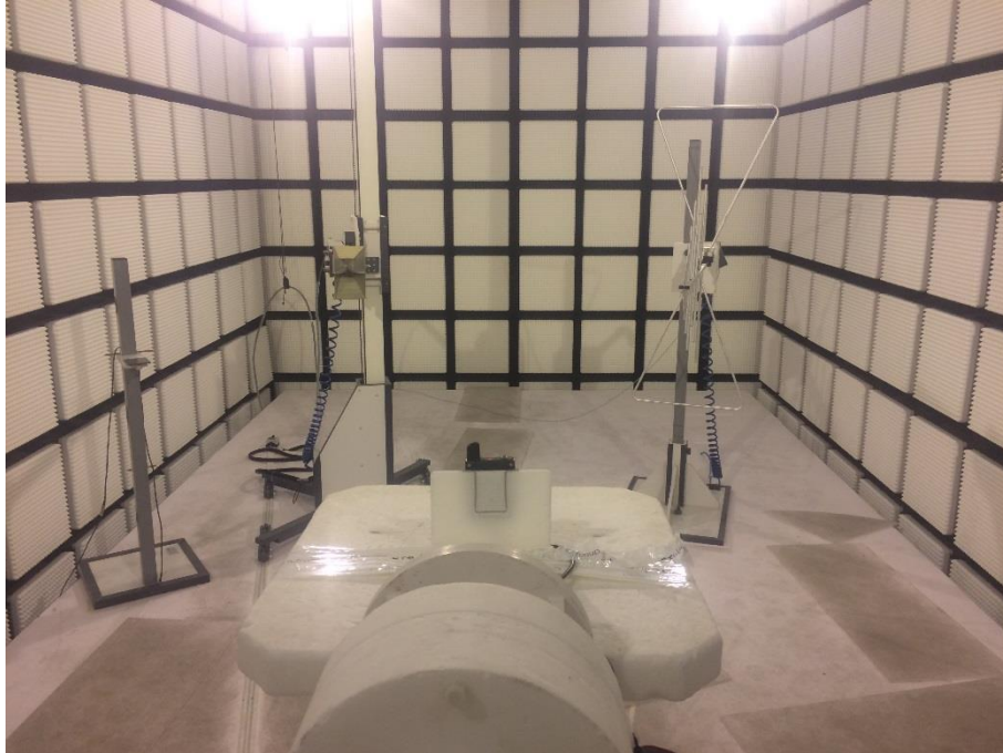
Photo 3: RSE set-up (>1GHz)
