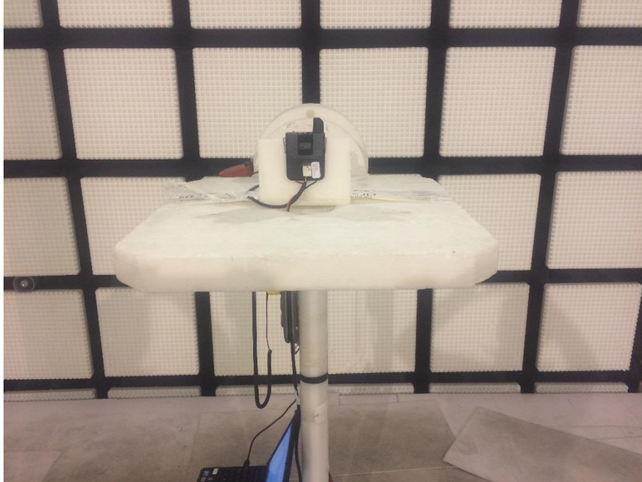
Photo 1: RSE set-up (>1GHz)
