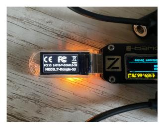
After connecting USB to power on. The screen can directly display the electronic label for two seconds.
