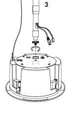
Plug in the Ethernet and 2-pin cables.
