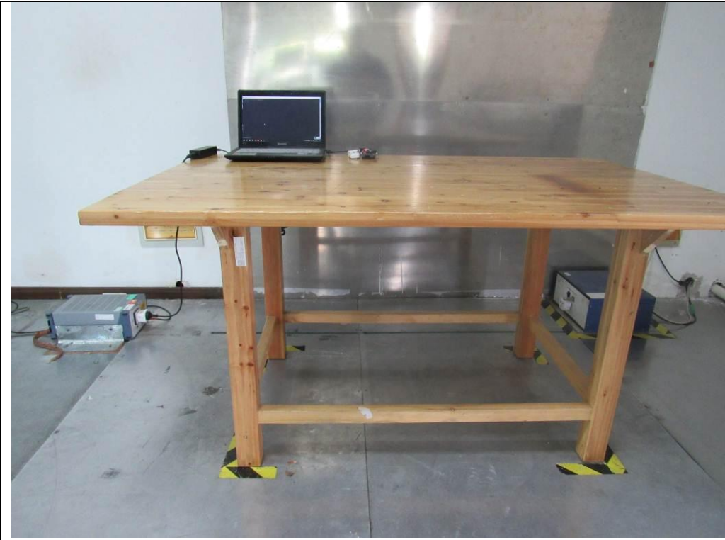
Conducted Emissions Test Setup – Front View
