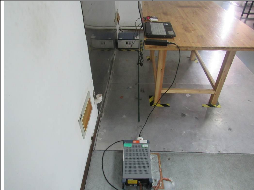
Conducted Emissions Test Setup – Rear View
