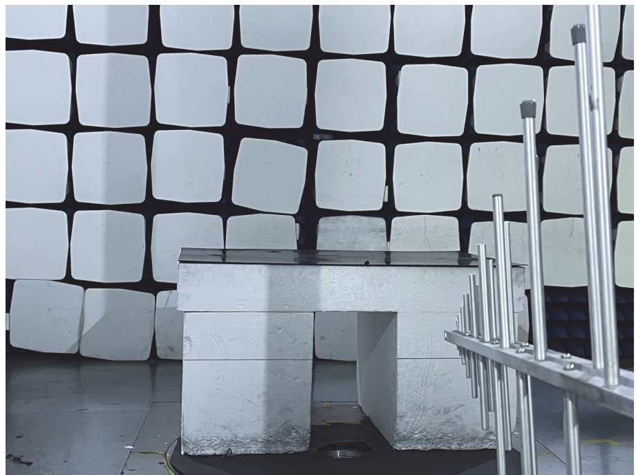
Radiation Emission Test Setup (30MHz to 1GHz)
