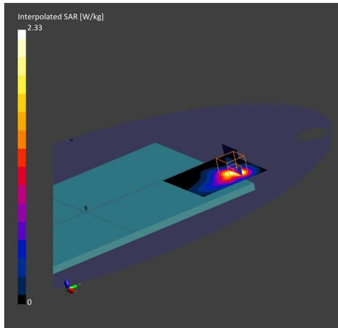
**10. LTE Band 38, QPSK - 20MHz, CH38150 – Back Face**
