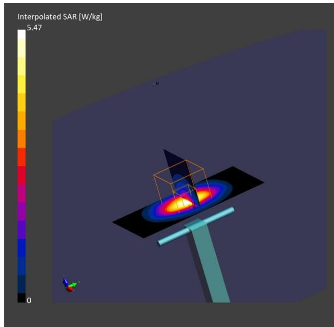
**21. System Check Body Liquid 2600MHz – 2021-03-19**
