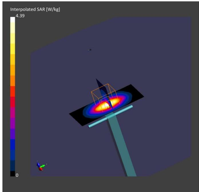
**20. System Check Body Liquid 2600MHz – 2021-03-18**
