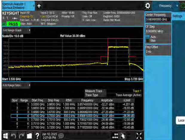
Plot 8-242. Channel Edge Emission Plot (n48_1C_30M_16QAM – High Channel_2T, Port 6)
