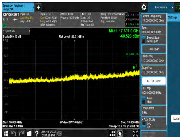
Plot 8-258. Conducted Spurious Emission Plot 10 GHz to 18 GHz (n48_2NC_40M+40M_QPSK - Mid Channel_2T, Port 3)
