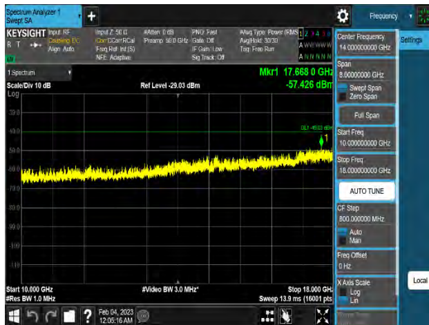
Plot 8-262. Conducted Spurious Emission Plot 10 GHz to 18 GHz (n48_1C_10M_QPSK - Mid Channel_8T, Port 8)
