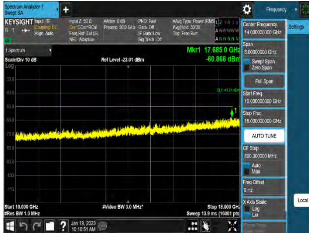
Plot 8-254. Conducted Spurious Emission Plot 10 GHz to 18 GHz (n48_2C_40M+40M_256QAM - Low Channel_2T, Port 4)
