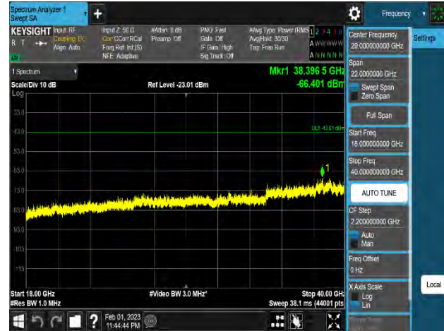
Plot 8-255. Conducted Spurious Emission Plot 18 GHz to 40 GHz (n48_2C_40M+40M_256QAM - Low Channel_2T, Port 4)
