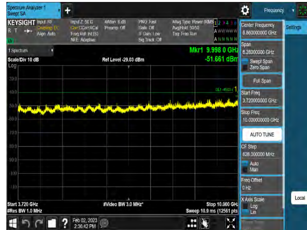
Plot 8-261. Conducted Spurious Emission Plot 3.72 GHz to 10 GHz (n48_1C_10M_QPSK - Mid Channel_8T, Port 8)
