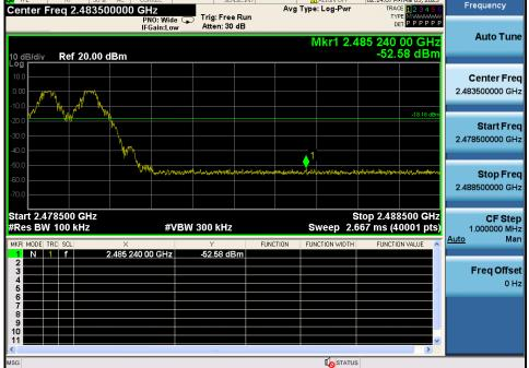
Conducted Spurious Emissions Highest Channel & Modulation : GFSK
