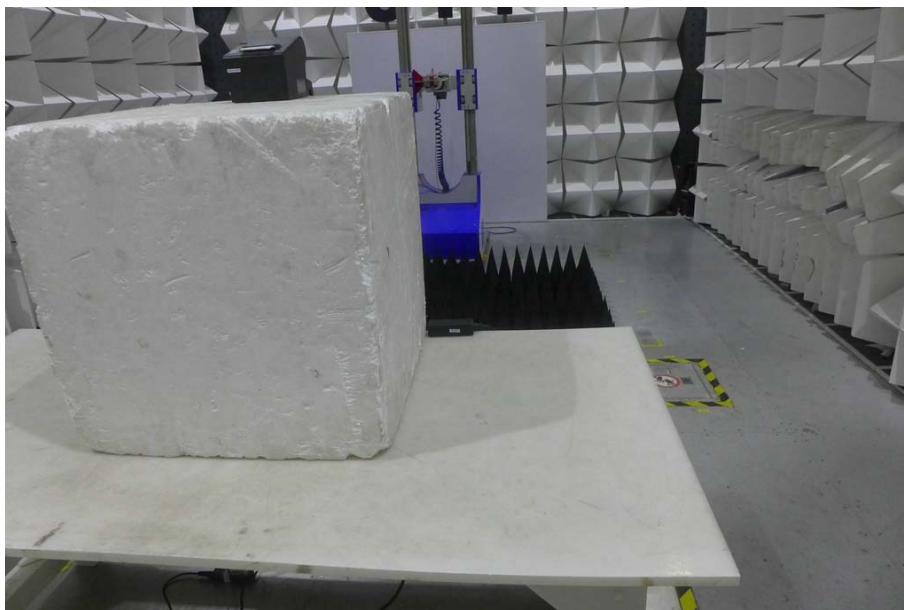
Radiated spurious emission Test Setup-3(Above 1GHz)
