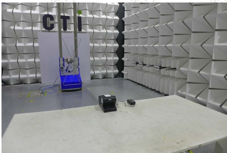
Radiated spurious emission Test Setup-2(30- 1000MHz)
