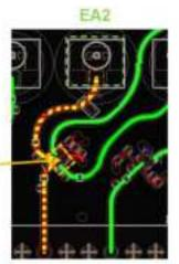
Trace Length: 599.88mil Trace Width: 12.5mil PCB thickness: 1.6mm Dielectric constant: 4 (FR-4) Trace copper foil : 1oz
