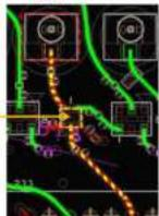
Trace Length: 495.74mil Trace Width: 12.5mil PCB thickness: 1.6mm Dielectric constant: 4 (FR-4) Trace copper foil 1oz
