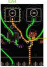
RF Switch Insertion Luse: 0.3 db @ 900 MHz 0.33 dB @ 1.8 GHz 0.37 dB @ 2.7 GHz 0.42 dB @ 4.2 GHz
