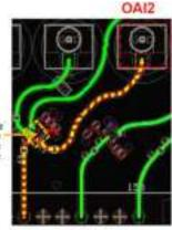
Trace Length, 744,34mil Trace Width: 12.5mil PCB thickness: 1.6mm Dielectric constant: 4 (FR-4) Trace copper foll: toz
