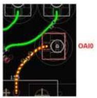
Trace Length: 360.36mil Trace Width: 12.5mil PCB thickness: 1.6mm Dielectric constant: 4 (FR-4) Trace copper foil: 1oz
