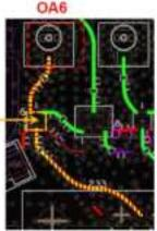
Trace Length: 627.04mil Trace Width: 12.5mil PCB thickness: 1.6mm Dielectric constant: 4 (FR-4)
