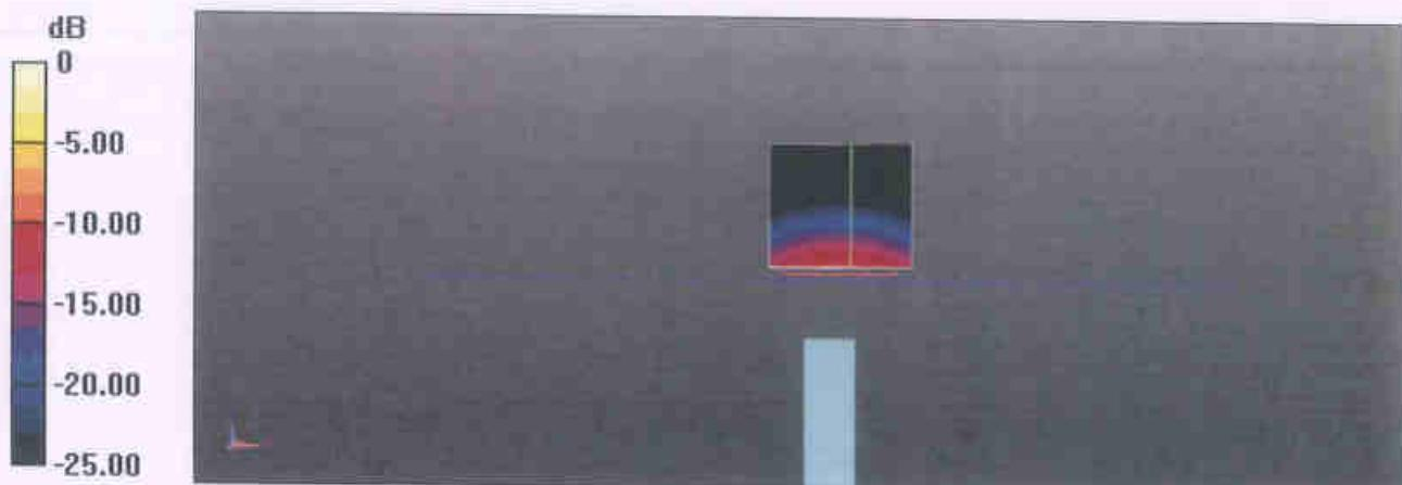
$$0 \text{ dB} = 17.8 \text{ W/kg} = 12.52 \text{ dBW/kg}$$
