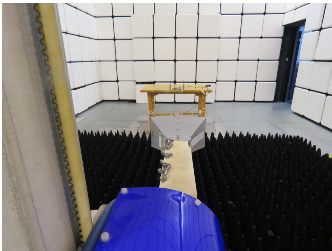
Picture 2: Radiated Spurious Emissions Test setup
